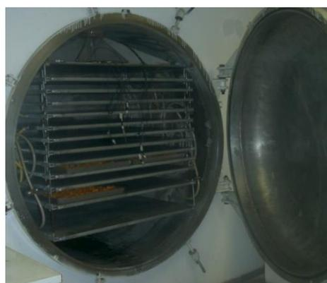
**Figure 1. Industrial lyophilising device with the additional parts**
