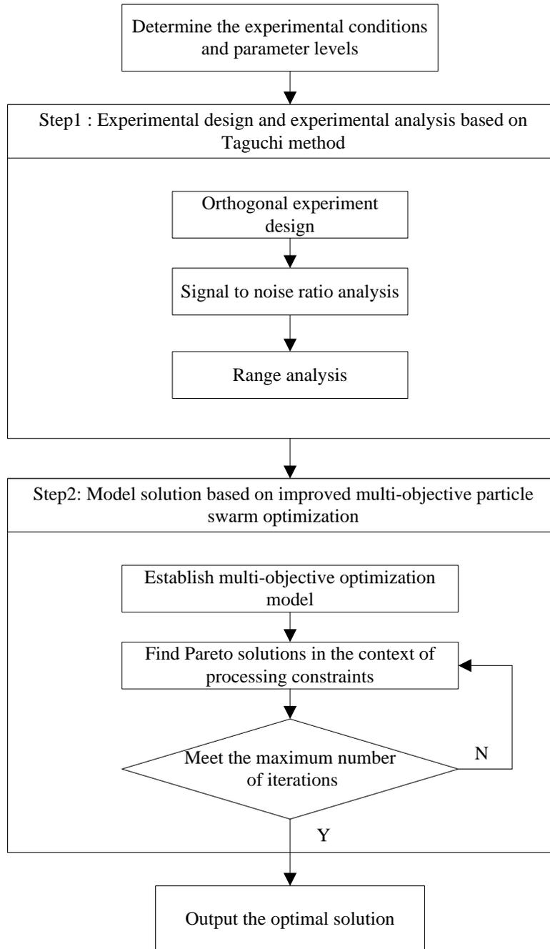
Figure 2. Flow chart of optimization method based on experimental data
