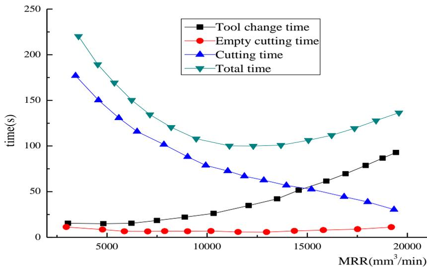
Figure 6. Time as a function of MRR for turning case
