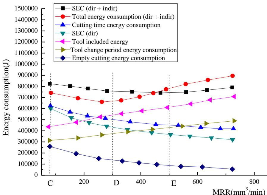
Figure 7. SEC as a function of MRR for milling case
