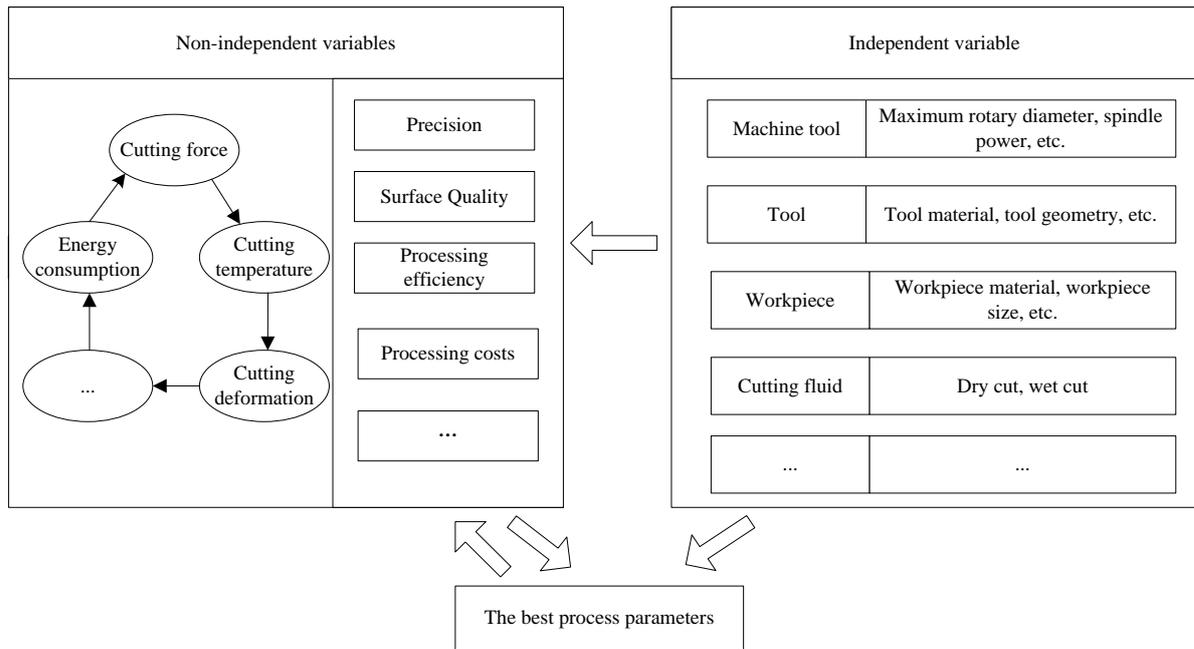
**Figure 1. Analysis of CNC machining variables**
