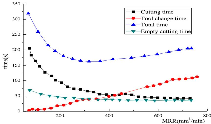
Figure 5. Time as a function of MRR for milling case
