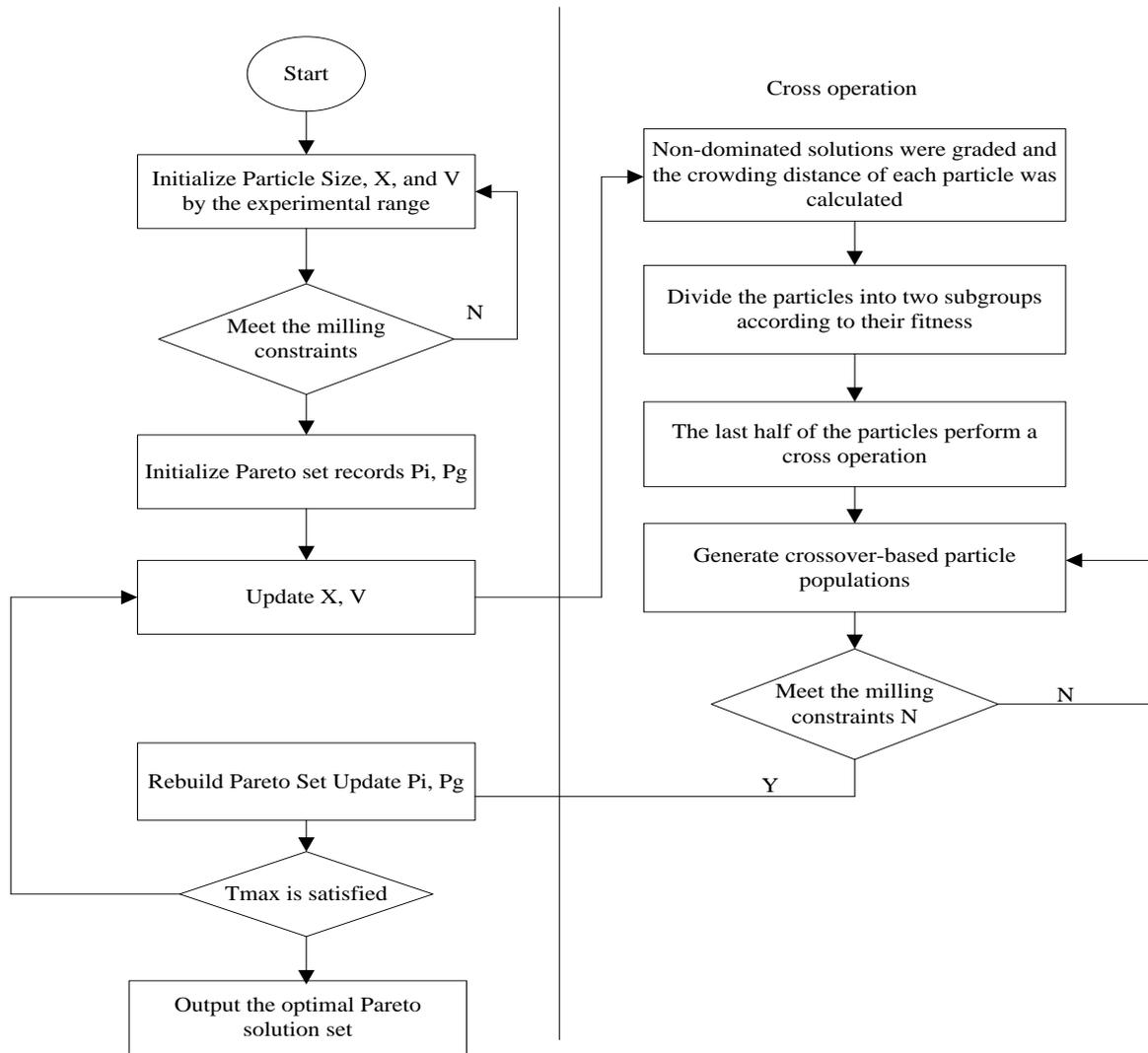
Figure 3. Flow chart of the MOPSO algorithm based on cross operation
