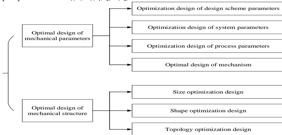
Figure 1. Common types of mechanical optimization problems
