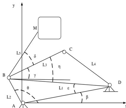
Figure 5. Four-bar mechanism
