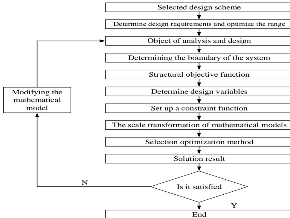
Figure 2. Optimization process diagram
