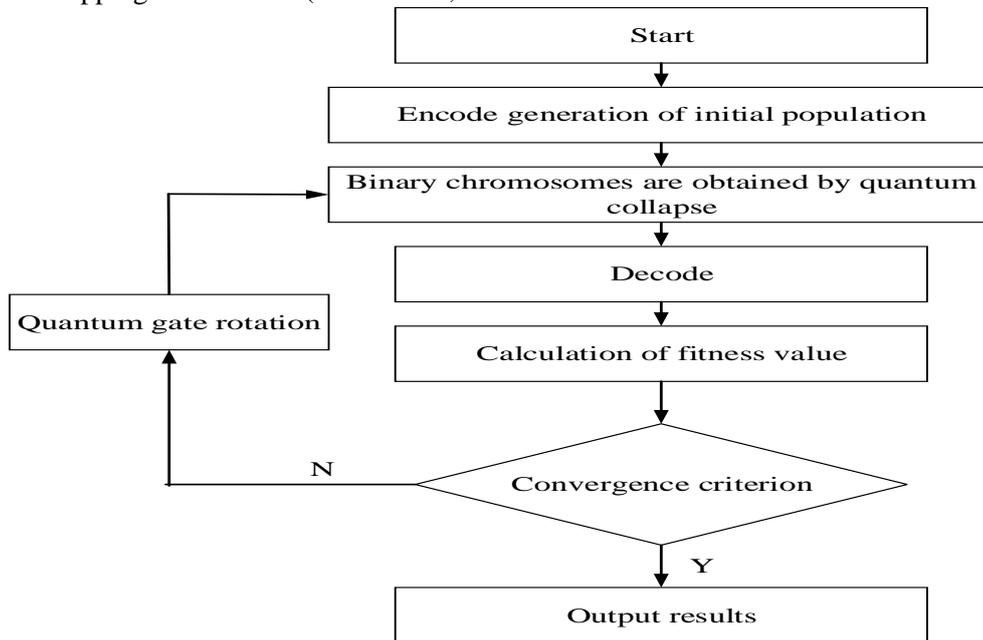
Figure 3. Quantum Genetic Algorithm Flow
