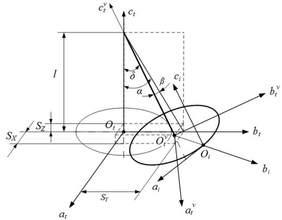
Figure 2 Transformation relation of cutter tooth cutting motion under vibration
