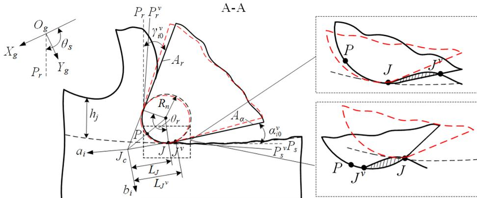
**Figure. 5 Friction pair of flank face under vibration**
