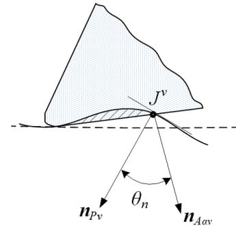
Figure. 6 Characteristic vectors of friction pairs under vibration
