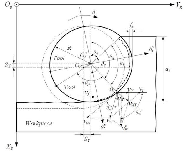
Figure. 7 Cutting motion mode and cutting speed decomposition of milling cutter
