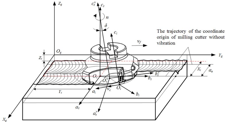
Figure 1. Coordinate systems of cutting motion of milling cutter
