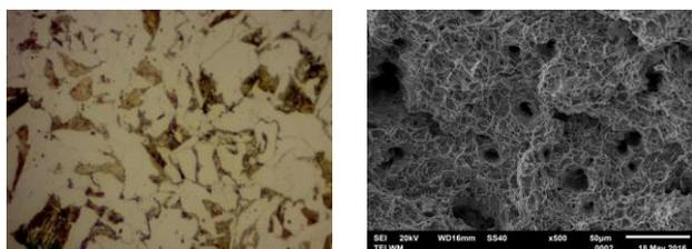
**Figure 3. Steel microstructure and the fracture surfaces observed using SEM showing manganese sulphide inclusions.**
