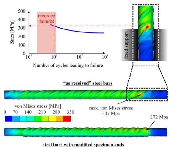
**Figure 7. Comparison of developing stress fields on the as received and treated bars.**
