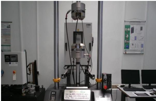
Figure 1. 100kN capacity Instron fatigue testing machine
