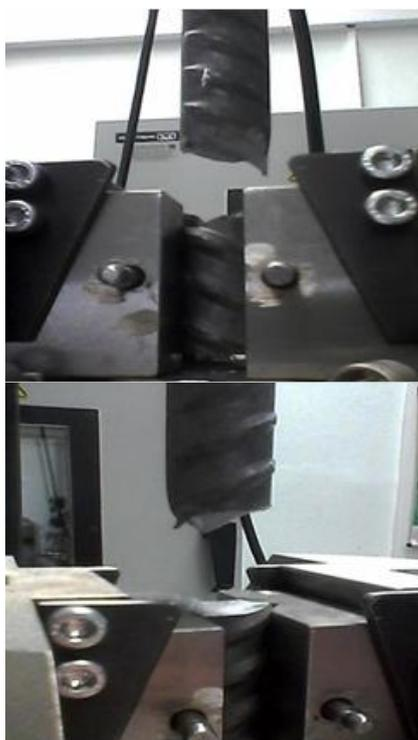
**Figure 2. Premature failure within or near grip jaws**
