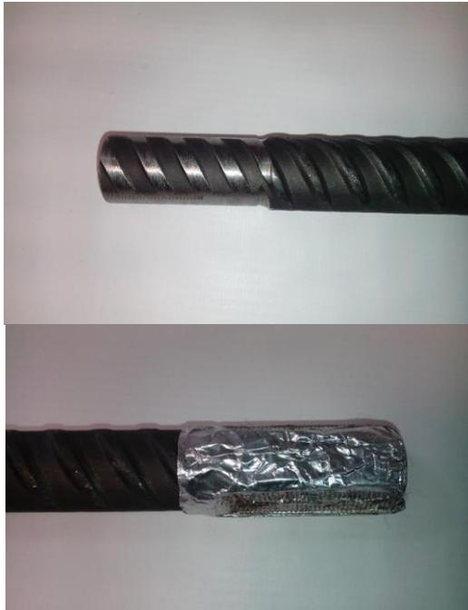
**Figure 4. Machined specimen ends and specimen ends wrapped with aluminium tape.**
