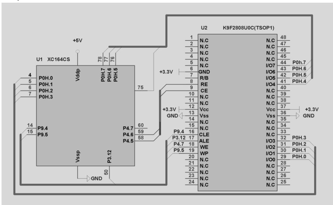
Figure 2 Interface Circuit between K9F2808U0C and XC164CS
