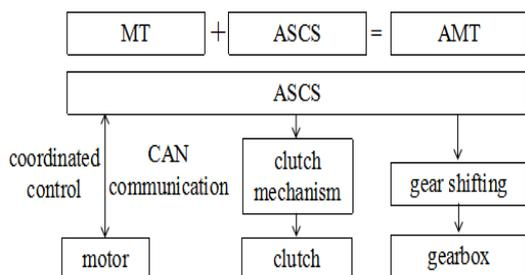
Figure 1 AMT Function Diagram of AMT
