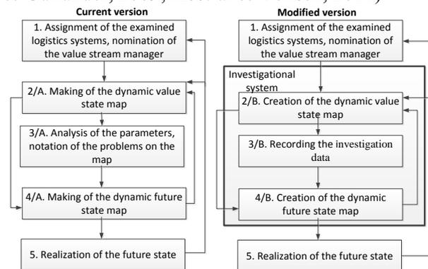
**Figure 3. Steps of the dynamic value stream mapping**
