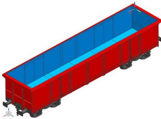
**Figure 7. The CAD model of the EAOS freight car with composite panels**
