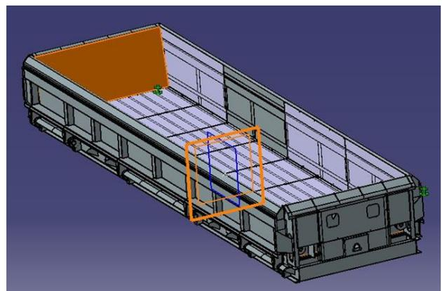
**Figure 6. Application of composite panels in the model of the type 418V of freight car**
