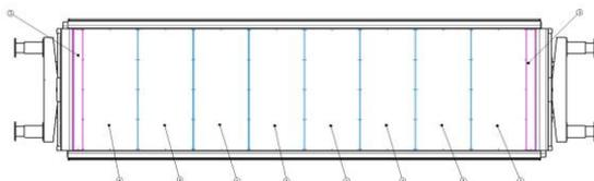
**Figure 8a. The distribution of composite panels to the shell of the 418V freight car body**
