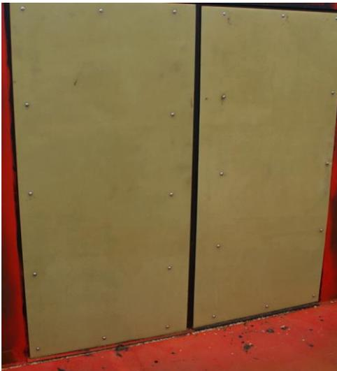
**Figure 10. Composite panels mounted on the freight car's doors**
