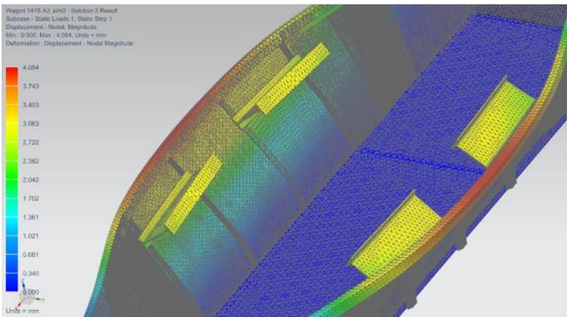
**Figure 3. Displacements of the freight car's body**
