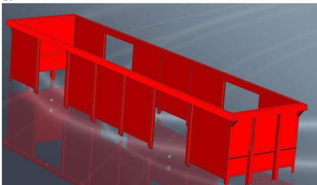
Figure 1. The CAD model of the freight car's body
