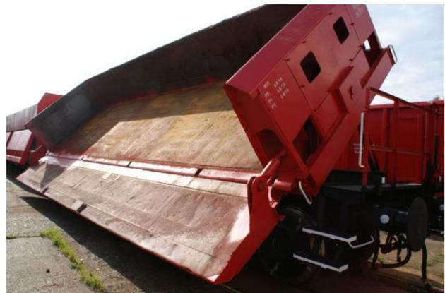
**Figure 5. The type 418V of the freight car**
