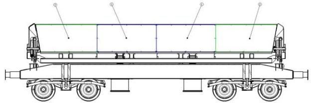
**Figure 8b. The distribution of composite panels to the shell of the 418V freight car body**
