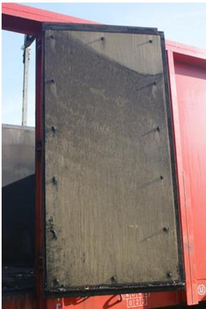
**Figure 11. The composite panel after exploitation**
