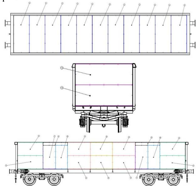
**Figure 9. The distribution of composite panels to the shell of the EAOS freight car body**
