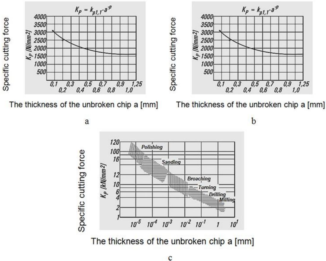
Fig.2 a,b,c. The dependence of the specific force on thickness of the unbroken chip (in linear an double logarithmic system) and the dependence  $K_p$
