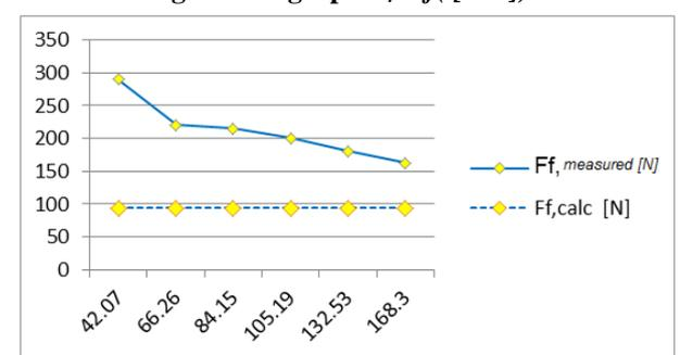
Fig. 4h The graph  $F_f = f(v[m/min])$
