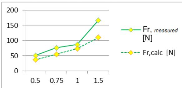
Fig. 4c The graph  $F_r = f(f[mm/rev])$
