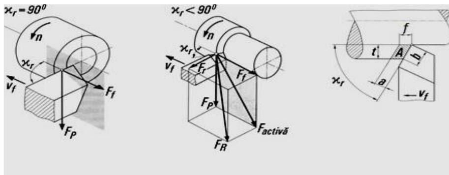
Technological parameters:  $t$  - depth of cut;  $f$  – feed rate
