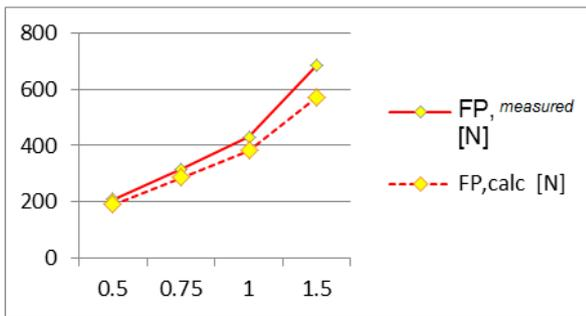
Fig. 4a The graph  $F_p = f(f[mm/rev])$
