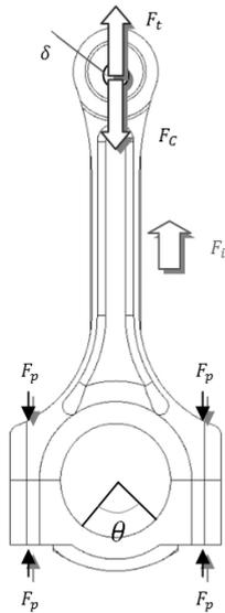
**Figure 1. Axial loads distribution on connecting rod's body.**
