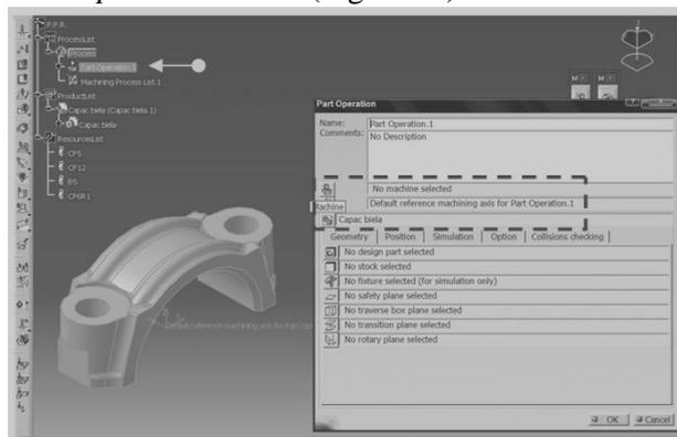
Figure 15. Part Operation menu for the connecting rod's head.
