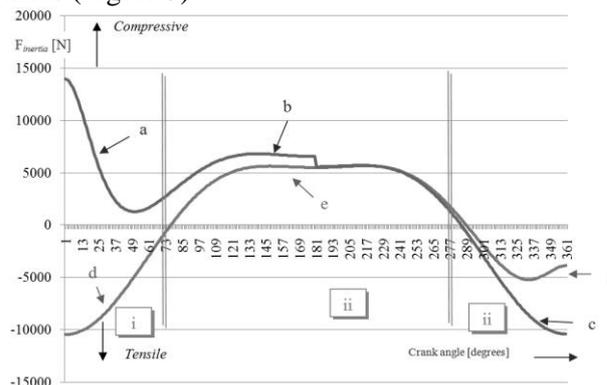
Figure 5. Inertia load distribution from  $0^\circ$  to  $360^\circ$  overlapped with the one from  $360^\circ$  to  $720^\circ$ .
