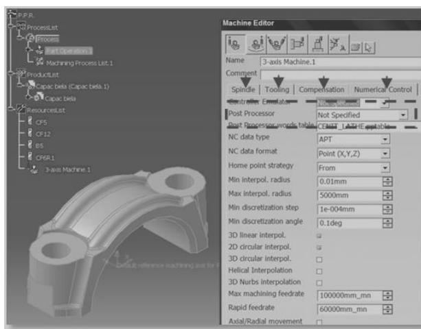
Figure 16. Post Processor definition menu for the connecting rod's head.
