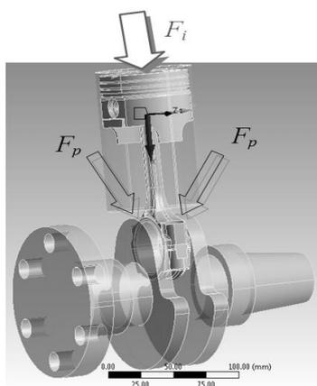
Figure 4. The assembly: the connecting rod, the piston and the crank.
