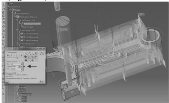
Figure 13. Roughing the connecting rod's body.
