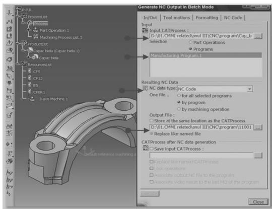
Figure 17. G type NC Code generation for the connecting rod's head.
