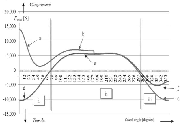
**Figure 2. Axial load distribution from 0° to 360° overlapped with the one from 360° to 720°.**
