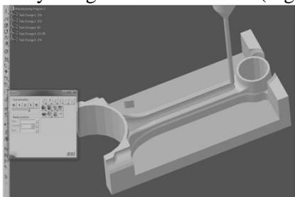
Figure 14. Z leveling the inner channels of the connecting rod's body.
