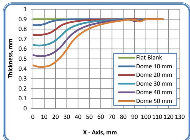
Figure 5. Thickness distribution of deformed dome parts.
