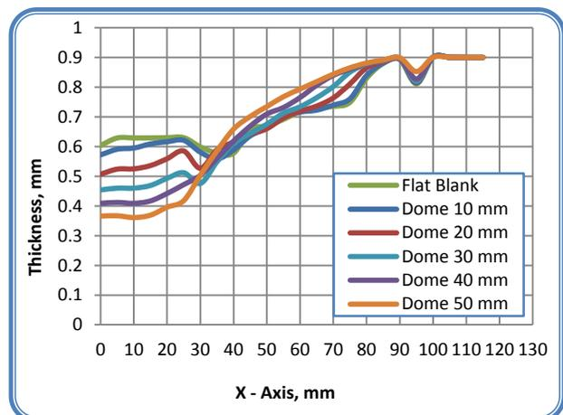
Figure 6. Thickness distribution of deformed SPIF parts.
