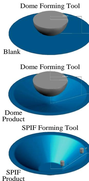
**Figure 3. Typical dome profiles and SPIF forming tool movement.**
