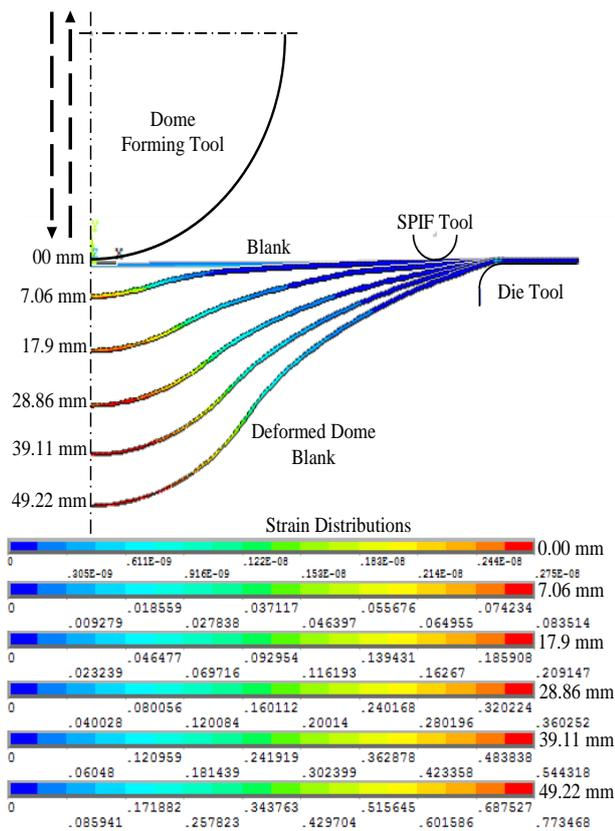
Figure 4. Typical Stress distributions stages of deformed dome parts.
