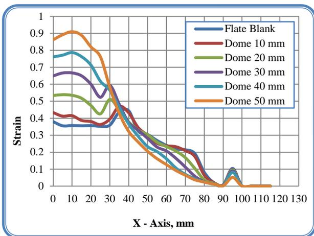
Figure 8. Strain distribution of deformed SPIF parts.
