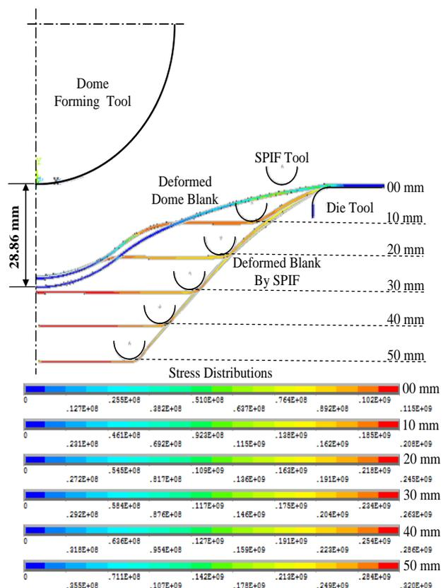
Figure 9. Stress distributions stages of deformed SPIF.
