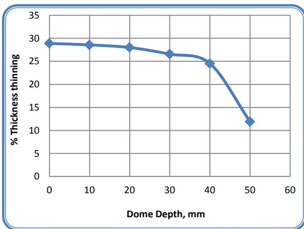
Figure 7. Thickness thinning of deformed blank.
