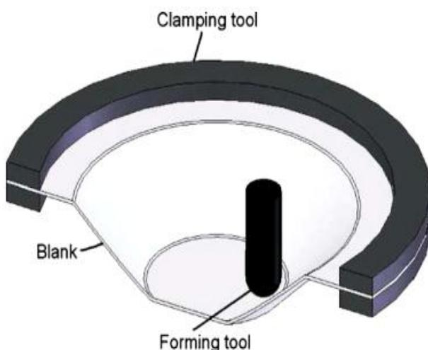
Figure 1. The basic component of SPIF process [1].
