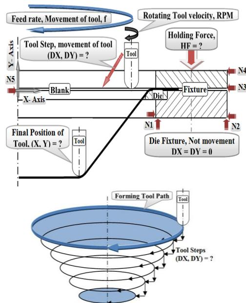
Figure 2. The basic component of SPIF process [1].
