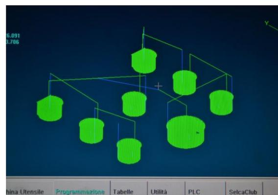
Figure 8. CNC simulation for injection mold machining –on FAMUP MC120 EVOLUTION
