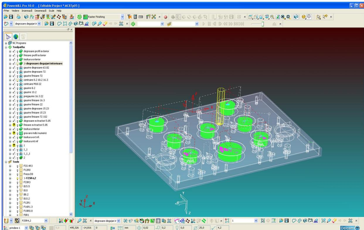
Figure 7. CAM simulation for a sequence of injection mold machining – PowerMill application
