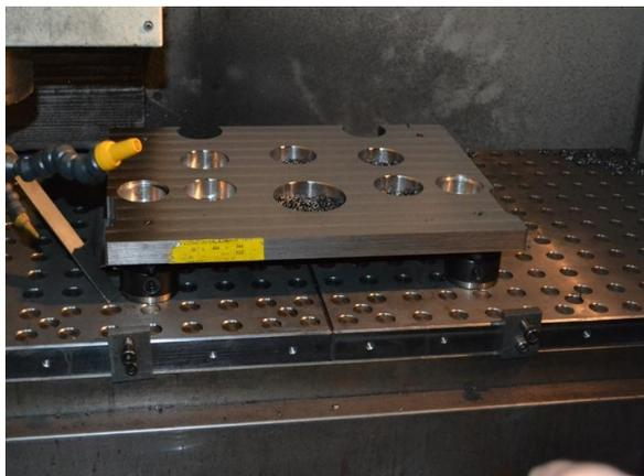
Figure 10. Injection mold part machined on FAMUP MC120 EVOLUTION
