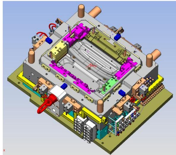
Figure 3. Complete CAD model for a complex injection mold – Cimatron application
