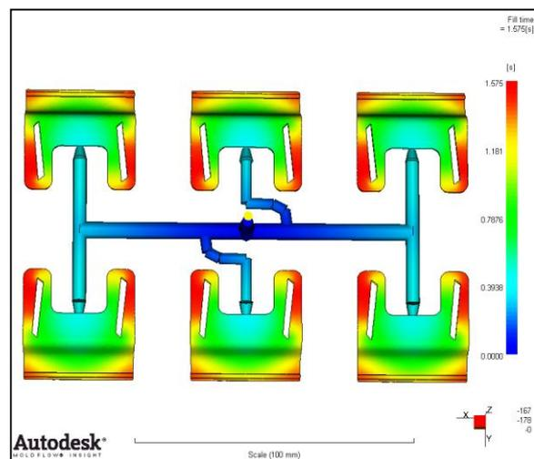
Figure 4. Injection molding process simulation – Autodesk Moldflow Insight application
