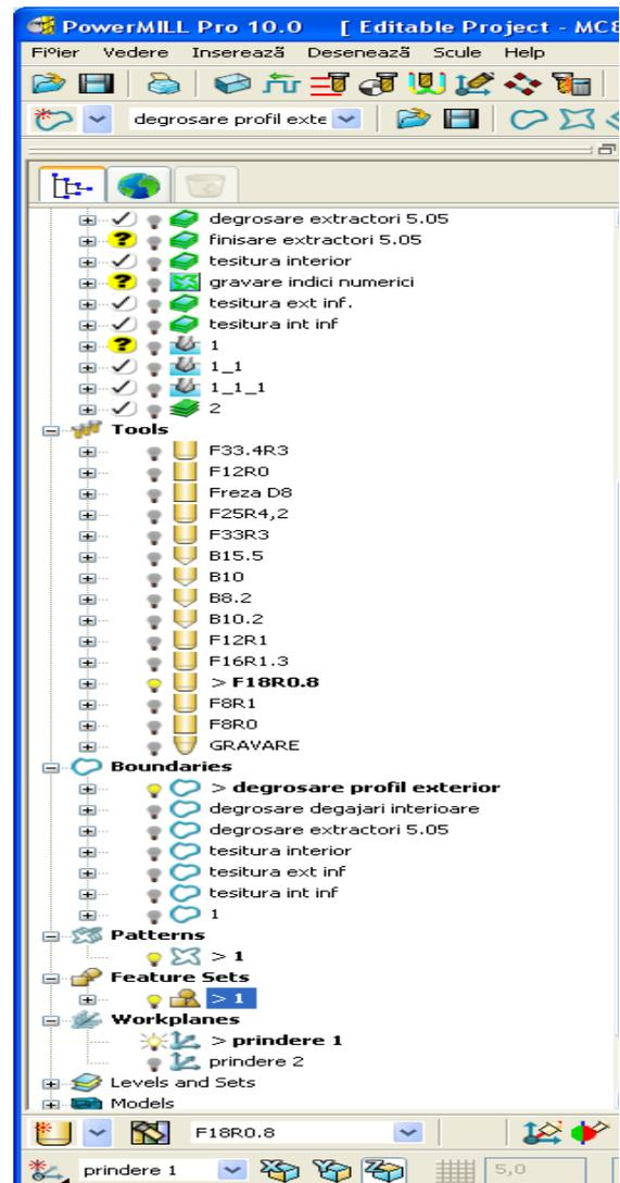
**Figure 6. CAM model for injection mold machining – PowerMill application**
