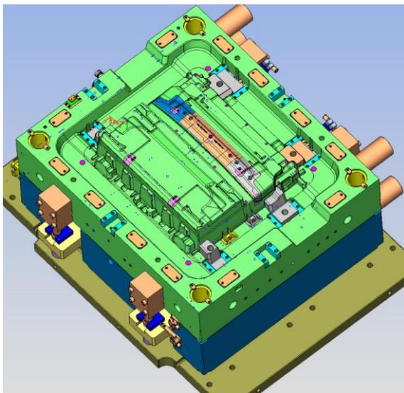
Figure 2. Partial model for a complex injection mold – SolidWorks application
