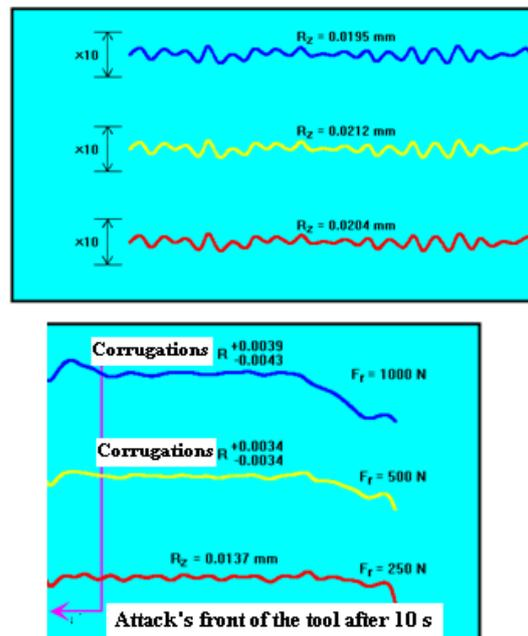
Figure 9. Machined surface profile depending on radial force
