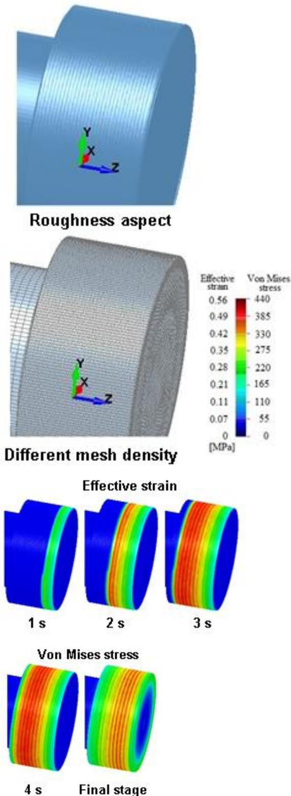
Figure 5. The workpiece discretization, effective plastic strain field and von Mises stress on active surface
