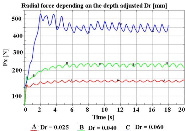
Figure 12. The radial force depending to the set depth Dr [mm]
