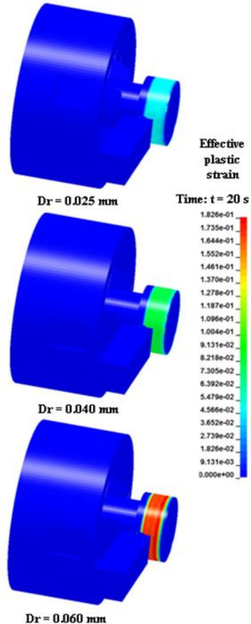
Figure 11. Effective plastic strain field at  $t = 20$
