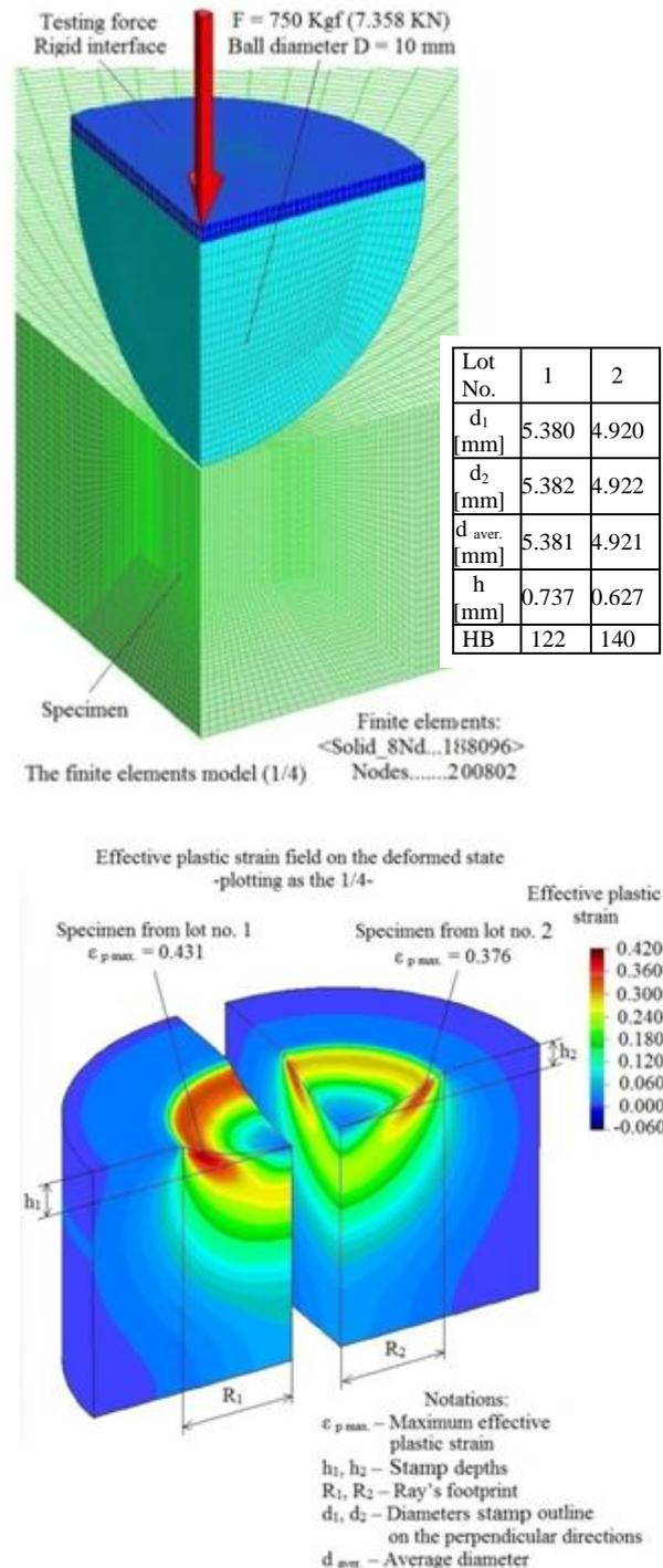
Figure 4. Brinell simulation test
