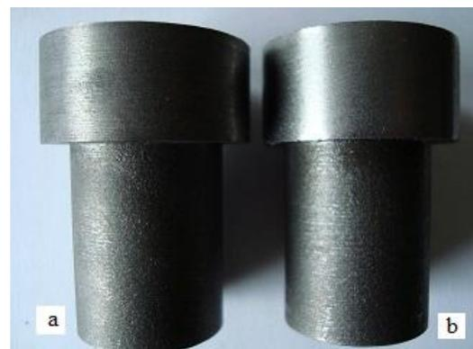
Figure 7. Workpieces a) before and b) after real smooth finishing
