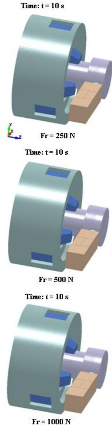
Figure 8. Qualitative analysis of machined surface depending on radial pressure force
