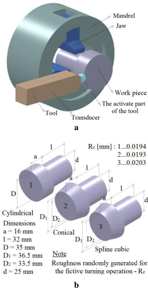
Figure 1. The physical model for the technological process of cold plastic deformation and workpiece model
