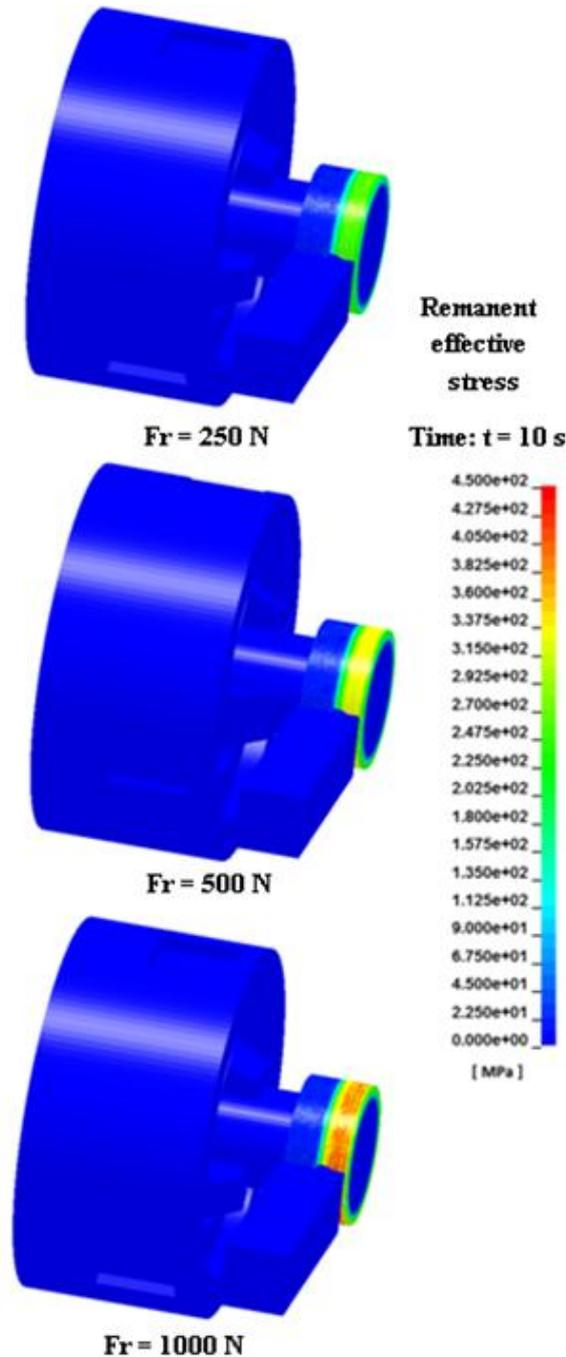
Figure 10. Remanent effective stress in the machined area after 10 s
