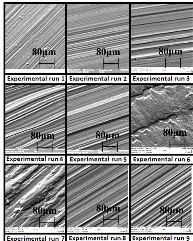
**Figure 5 SEM micrographs of the machined surface obtained in the experiments**
