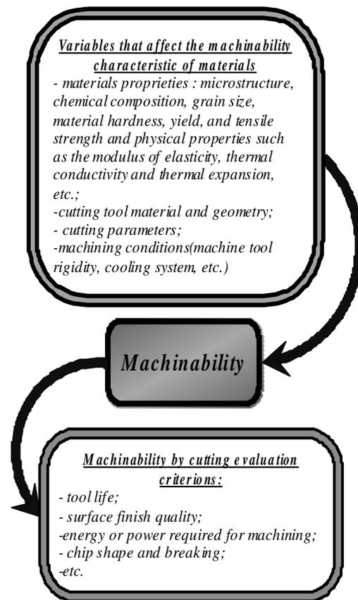
Figure 1 Material machinability characteristic analyze
