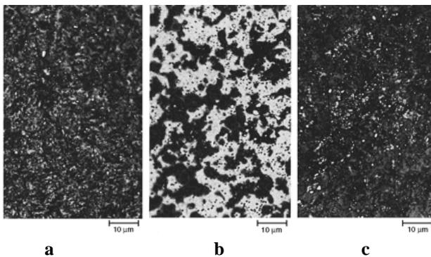
**Figure 2** AISI W1 (1.05% C), 19 mm diameter bars, brine quenched: (a) Hardened case microstructure. 64 HRC. Case contains as-quenched martensite and undissolved carbides. 4% picral; (b) Transition zone. 55 HRC. Martensite is light and undissolved, carbide is outlined, and pearlite is dark. 4% picral; (c) Core microstructure. 42 to 44 HRC. 4% picral etch reveals fine pearlite matrix (black) containing some patches of martensite (white) and undissolved carbides (outlined white particles). 1000x
