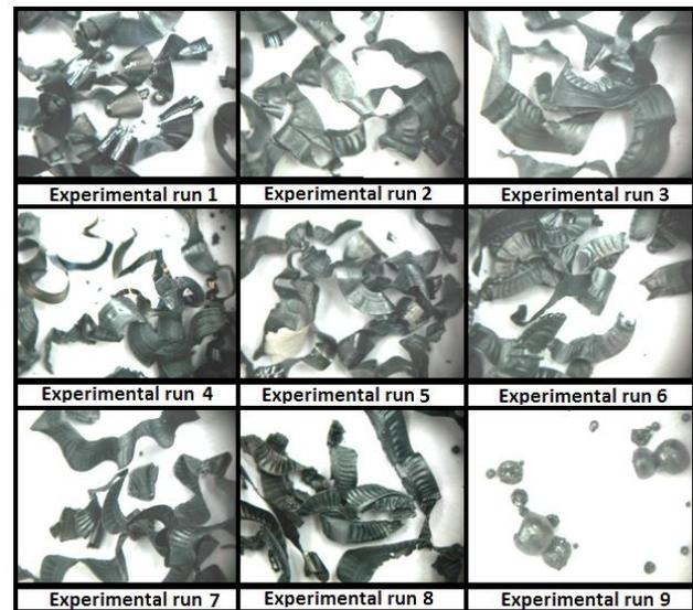
**Figure 4 Chip shapes obtained in the experiments 8X magnitudes**
