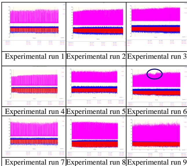
**Figure 3 Reports showing the cutting force components evolution during machining generated with Dynoware specialized software**
