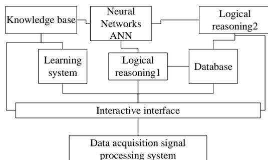
**Figure 1.** Block diagram of a serial connection method neural network fault diagnosis expert system
