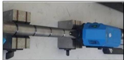
Fig.4. Roughness measurement of the sections with the Hommel T500
