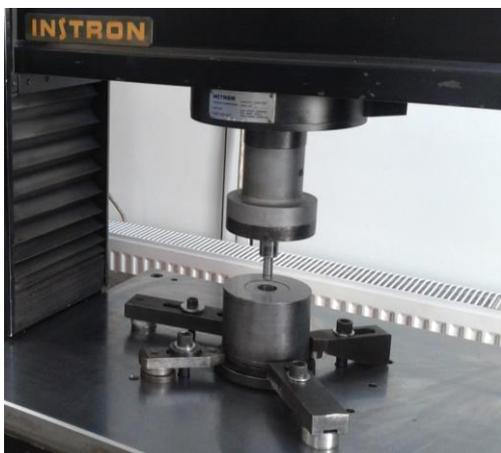
Figure 6. Experimental setup used for the combined forward conical can-backward straight can extrusion
