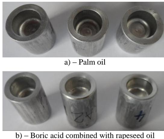
Figure 7. Extruded test specimens using different lubricants (punch stroke: 11 mm)
