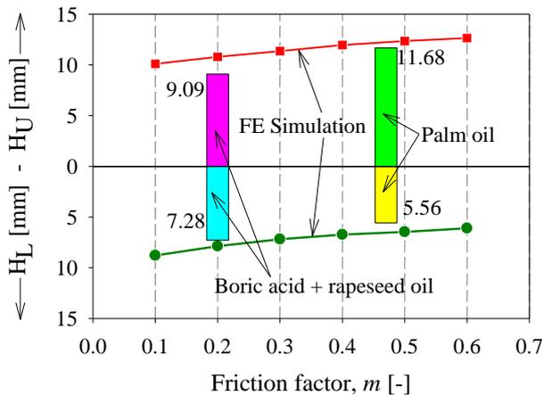
Figure 12. Friction calibration curves and experimental results (punch stroke: 11 mm)
