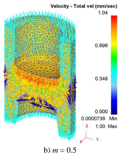
**Figure 11. Effect of friction factor on the material flow (punch stroke: 11 mm)**
