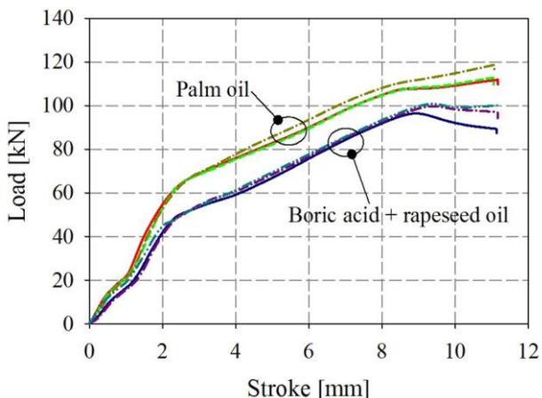
Figure 13. Load-stroke curves for two friction conditions
