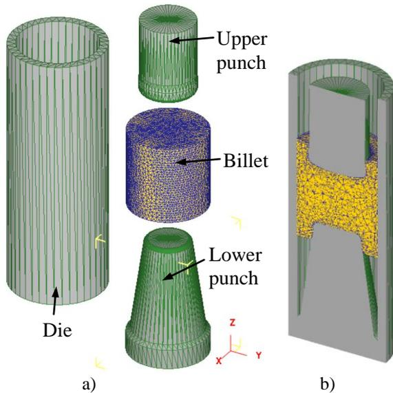
**Figure 8. FE simulation model of combined forward conical can-backward straight can extrusion test: a) – components of the FE model; b) – during the FE simulation**
