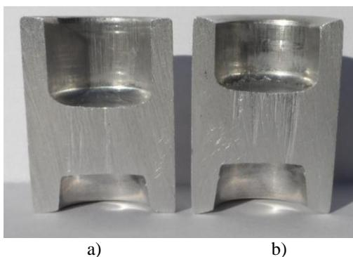
**Figure 9. Axial section of the test specimens extruded in different friction conditions: a) - palm oil; b) – boric acid combined with rapeseed oil (punch stroke: 11 mm)**
