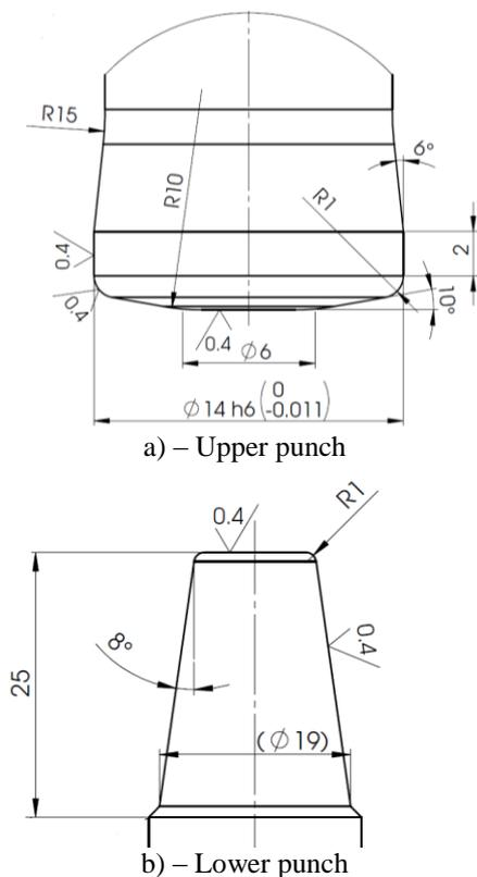
Figure 5. The shape and the main dimensions of the punches
