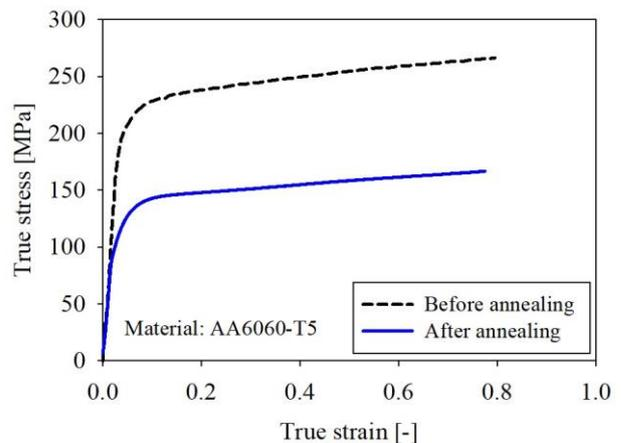
**Figure 4. True stress – true strain curves**
