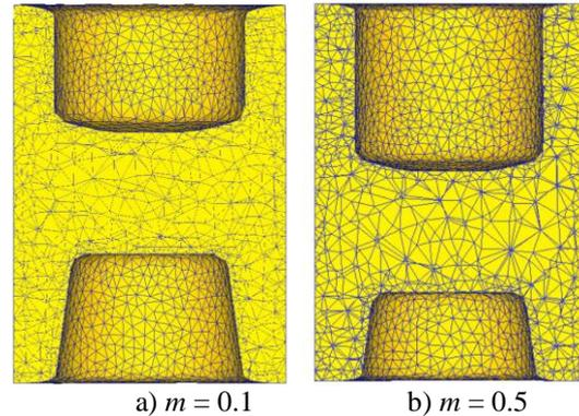
**Figure 10. FE simulation extruded billets for two values of friction factor ( $m$ ) (punch stroke: 11 mm)**
