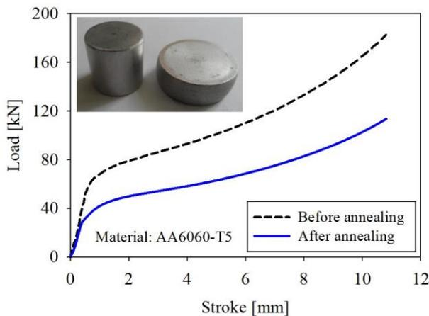
**Figure 3. Load - stroke curves during the uniaxial compression test**
