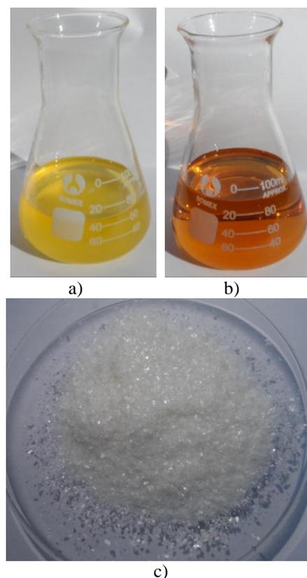
Figure 2. Lubricants: a) – palm oil; b) – rapeseed oil; c) – boric acid
