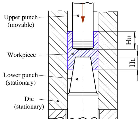
Figure 1. Schematic representation of material flow during the combined forward conical can-backward straight can extrusion test
