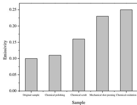
**Figure 2** Surface radiation rate of each sample
