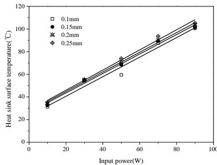
Figure 5 The surface temperature of the heat sink varies with the thickness of the coating after the correction
