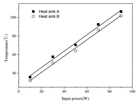
**Figure 4** The experimental data of heat sink after the correction
