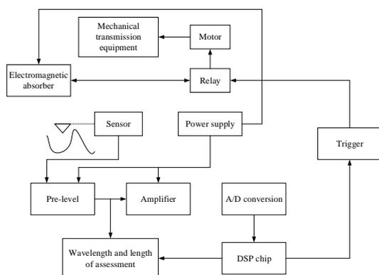
Figure 1 Flow chart of roughness instrument
