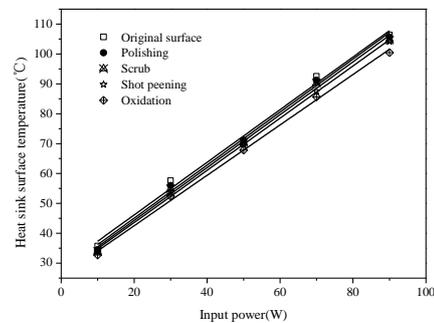
Figure 7 impact of surface roughness on the heat sink temperature
