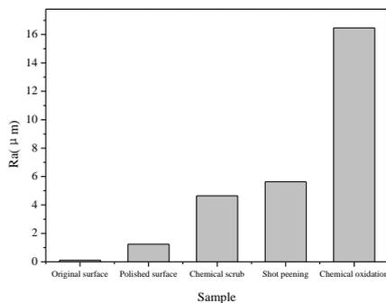
Figure 6 Ra value of surface of heat sink after different surface treatments
