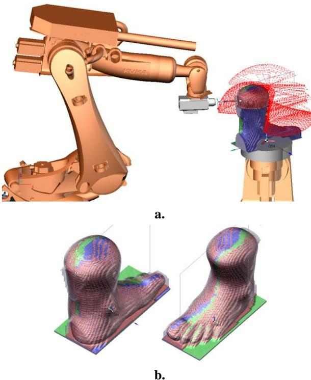
**Figure 12. Screenshot from rotary machining simulation(a); final part (b)**
