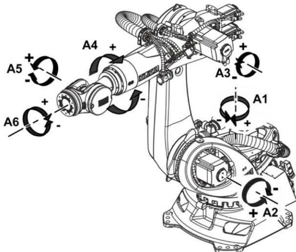
Figure 6. KUKA six axes serial robotic structure (source KUKA AG company website)
