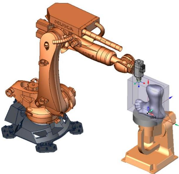
Figure 9. 3D model of the robotic cell, workpiece and machined part
