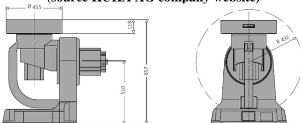
Figure 7. KUKA DKP 400 positioning unit (source KUKA AG company website)
