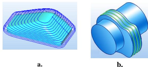
Figure 10. Roughing waterline strategy (a); rotary machining strategy (b)
