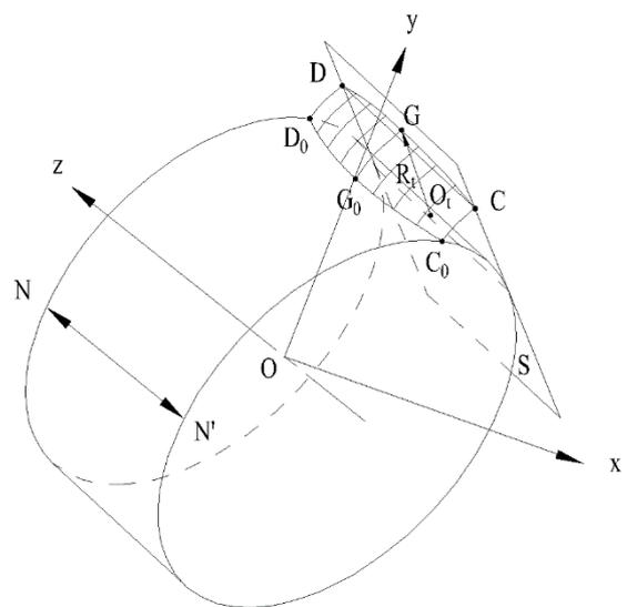
**Figure 1. Generation of the tooth surface of the IAGD**
