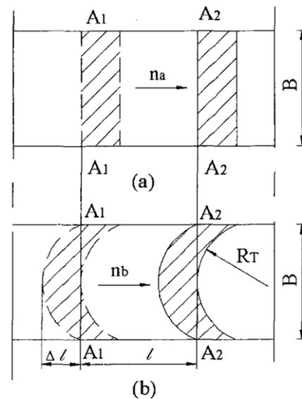
Figure 3. Contact ratio calculation of the IAGD
