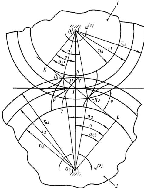
Figure 2. Random radial crosssection of involute gear meshing
