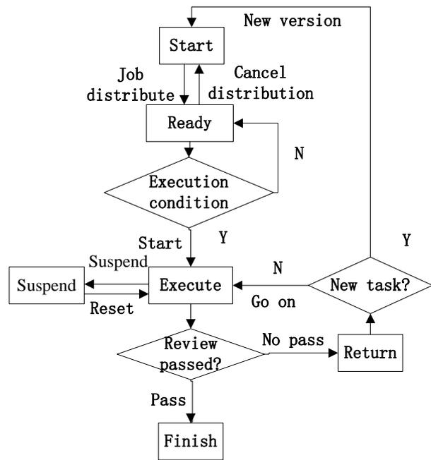
Figure 2. The execution state change model of production process
