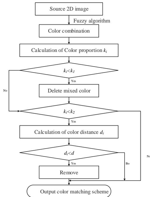
Figure 1. Extracting Process of Color Matching Scheme
