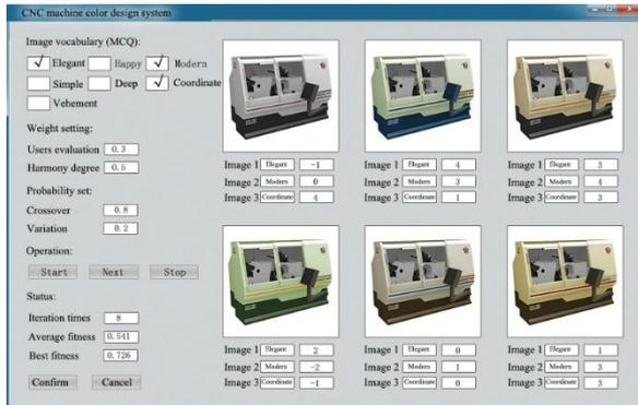
**Figure 4. CNC machine color design interactive genetic operation interface**
