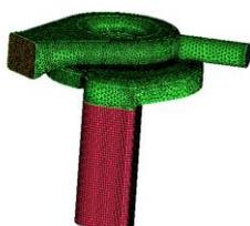
Figure 2. Mesh model for the centrifugal pump
