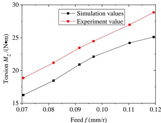
Figure 11. Cutting force comparison of 20CrMnMo
