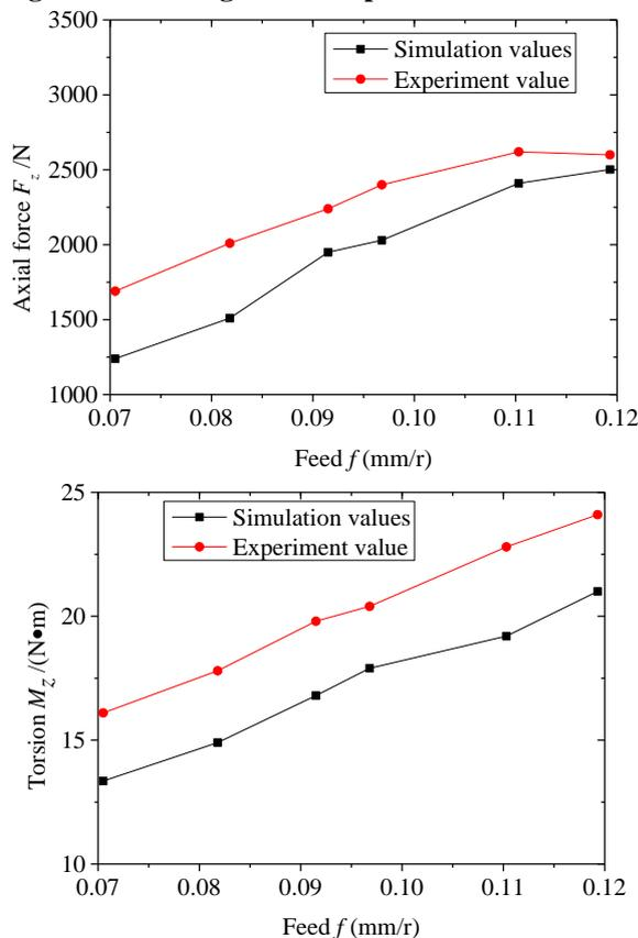
Figure 12. Cutting force comparison of 45 steel
