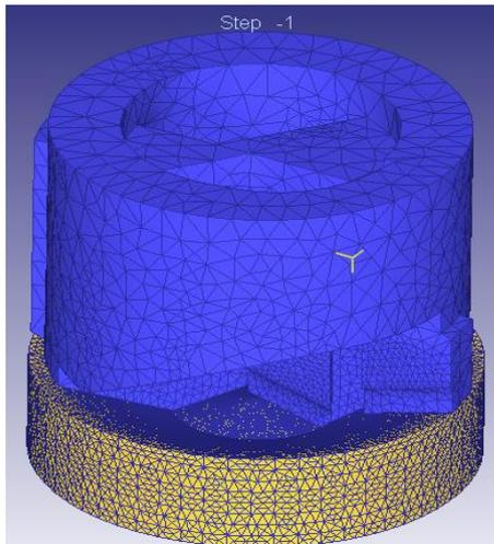
Figure 4. Finite element simulation model and grid division
