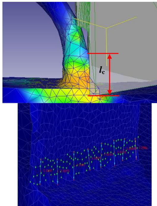
**Figure 7. The length measurement chart of the tool-chip contact**
