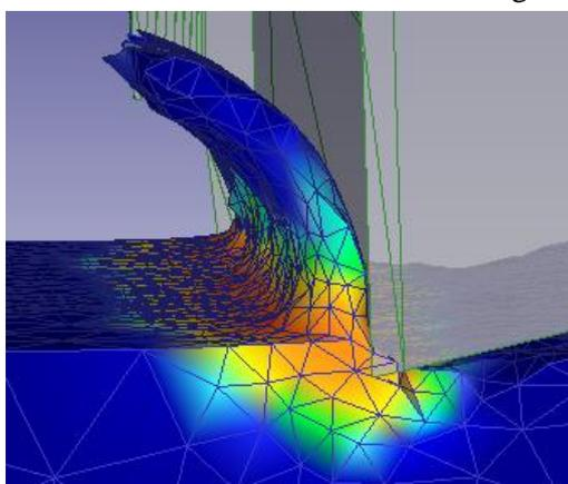
Figure 5. The simulation results of chips forming process
