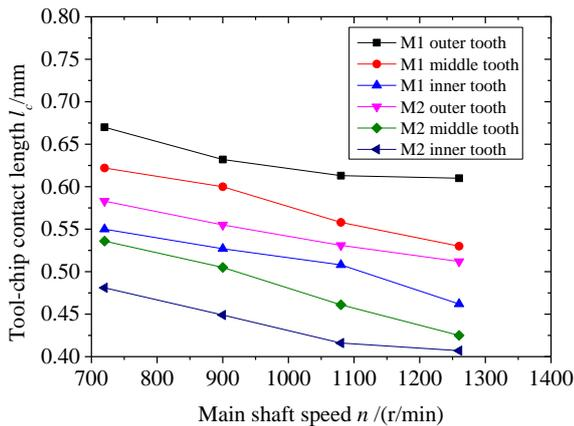
**Figure 9. Tool-chip contact length  $l_c$  vs. main shaft speed  $n$**
