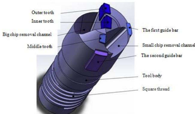
**Figure 2. Graphic model of staggered teeth BTA drill**
