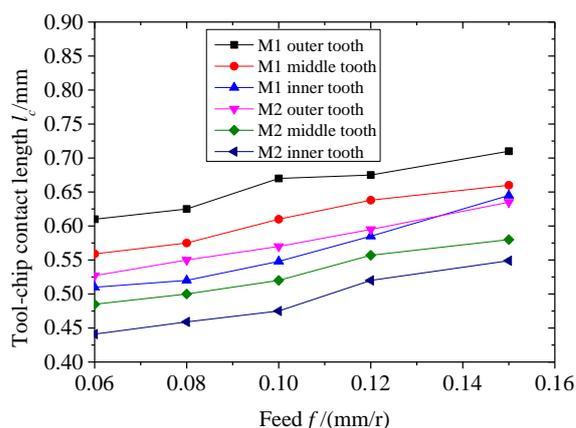
**Figure 8. Tool-chip contact length  $l_c$  vs. feed  $f$**
