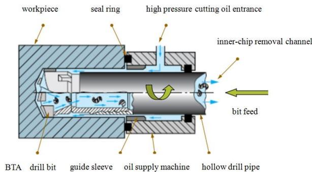
**Figure 1. Operating principle of the BTA deep-hole machining system**
