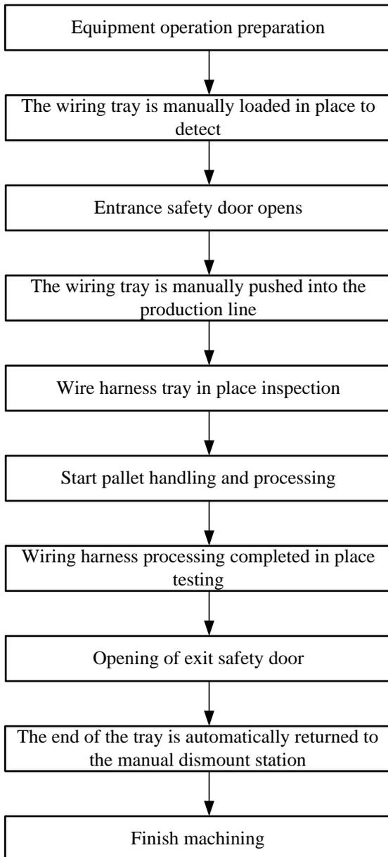
Figure 3. Main action flow chart of production line
