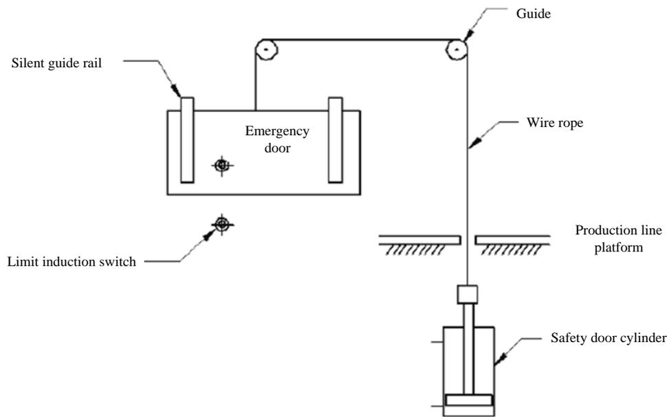
Figure 5. Schematic diagram of entrance safety door and exit safety door
