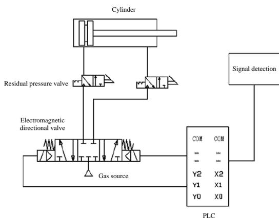
Figure 6. Safety door control principle diagram
