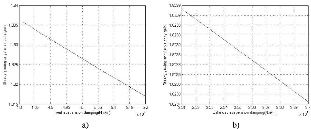
**Figure5. Relationship between steady-state yaw rate gain and front suspension or equilibrium suspension damping**
