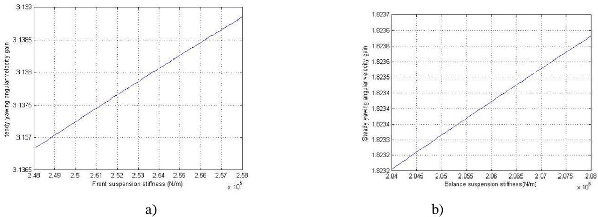
**Figure4. Relationship between steady-state yaw speed gain and front suspension or equilibrium suspension stiffness**
