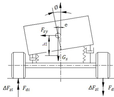
Figure2. A diagram of the force on the side of the vehicle
