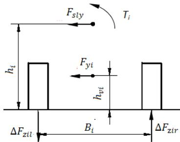
**Figure 3. The schematic diagram of three axis lateral reaction force**
