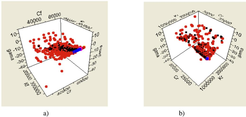
**Fig. 7 Pareto optimal solution set of front suspension or equilibrium suspension stiffness and damping (for the roll stability)**
