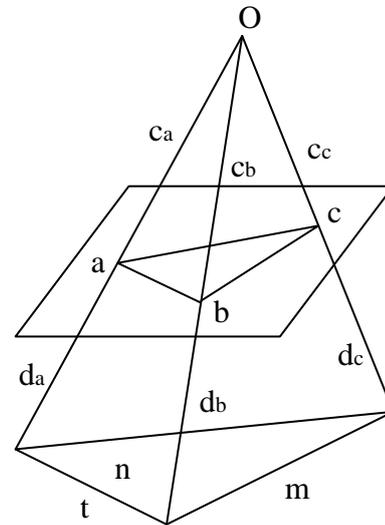
**Figure 5.** P3P principle
