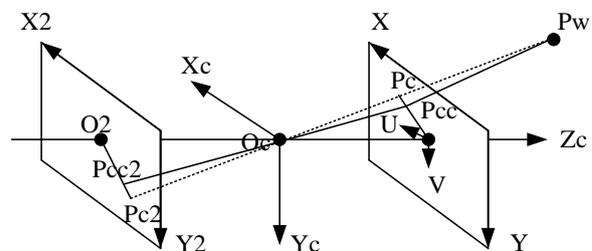
Figure 2. Perspective projection imaging model
