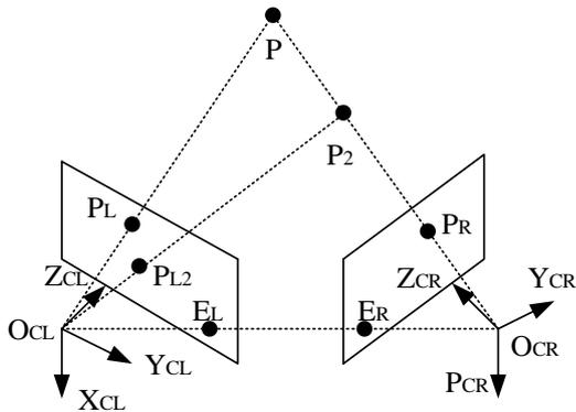
**Figure 3.** Binocular vision imaging model
