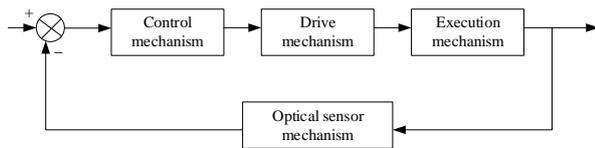
**Figure 4.** Schematic diagram of hardware structure
