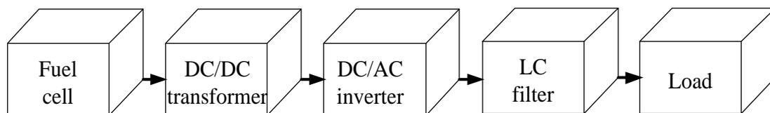
Fig.1 System structure diagram of solid oxide fuel cell generator
