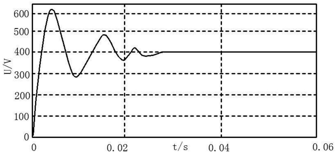
Fig.5 DC bus voltage of the Boost converter circuit
