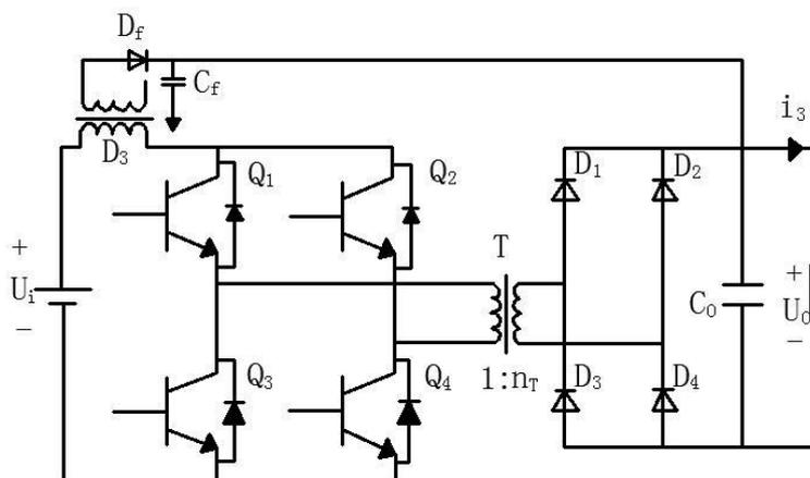
Fig.2 Improved DC/DC converter
