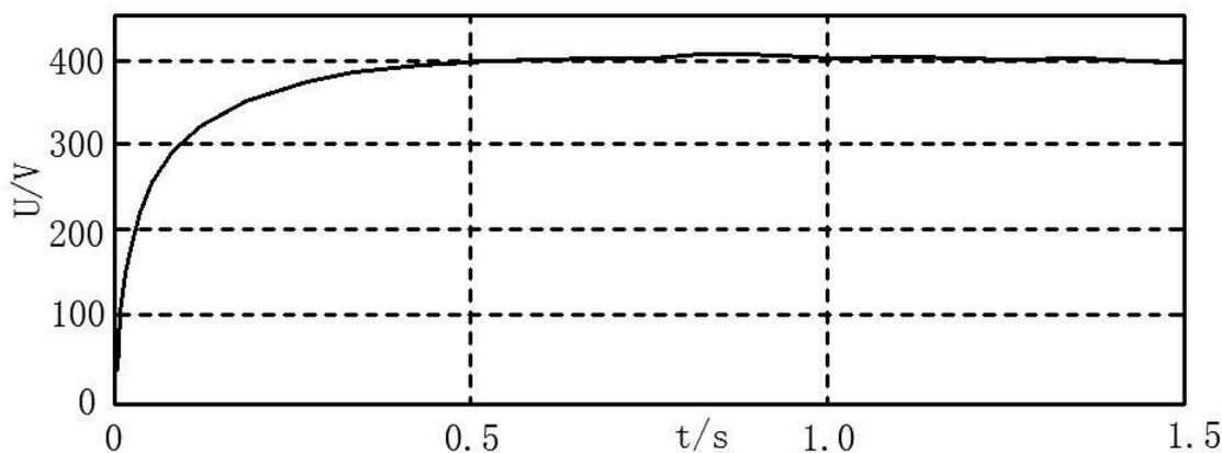
Fig.6 DC bus voltage of isolated full-bridge inverter circuit
