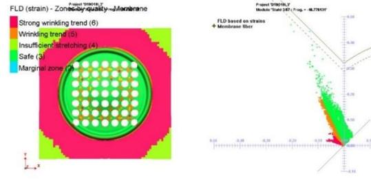
Figure 13. FLD Strain D10O10L0.3
