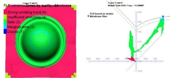
Figure 3. Validated FLD using PAMSTAMP (friction coefficient 0.12 – lubricated condition).
