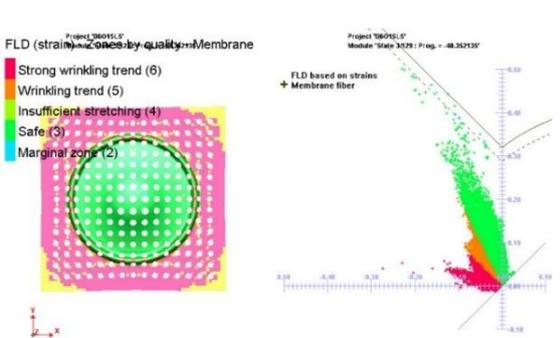
Figure 8. FLD Strain D6O15L0.5.
