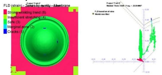
Figure 4. Validated FLD using PAMSTAMP (friction coefficient 0.3- dry condition)
