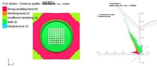
Figure 6. FLD Strain D6O5L0.3
