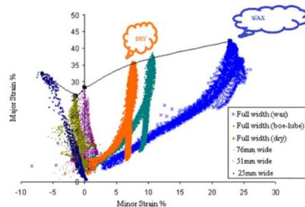
Figure 5. FLD used for validation from AlaHijazi et al 2004 [27] Experiment
