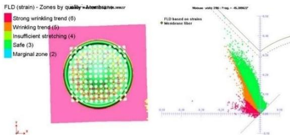
Figure 7. FLD Strain D6O10L0.4
