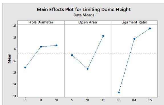
Figure 15. Main effects plot for limiting dome height
