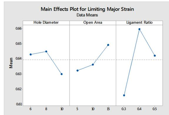
Figure 16. Main effects plot for limiting major strain
