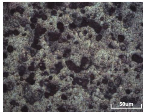
**Figure 2. Microstructure of robot laser hardened specimen.**
