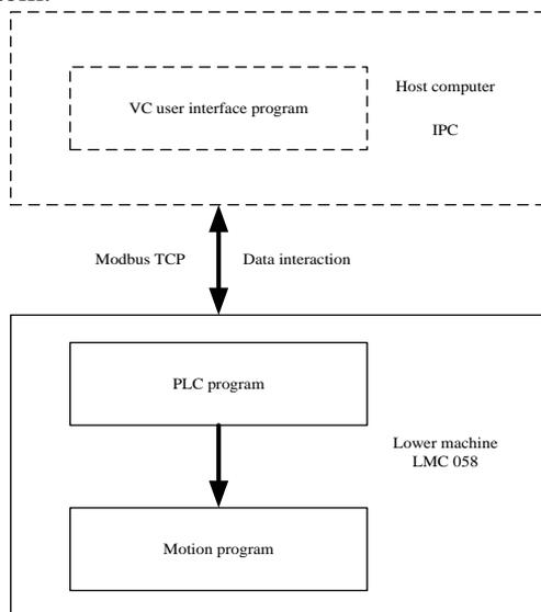
Figure 2. Software control system hierarchy
