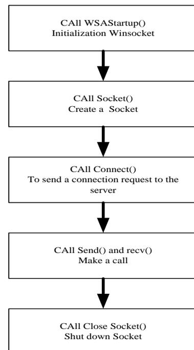
Figure 4. The flow chart of the client connecting with the server
