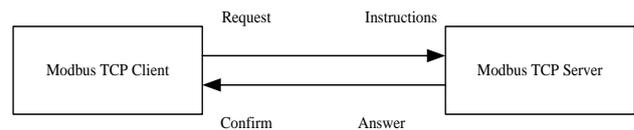
Figure 3. Modbus TCP network communication mode
