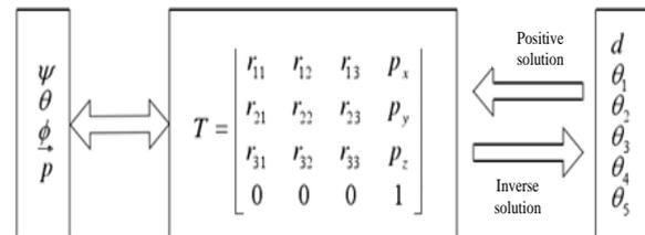
Figure 5. The process of positive and negative solution
