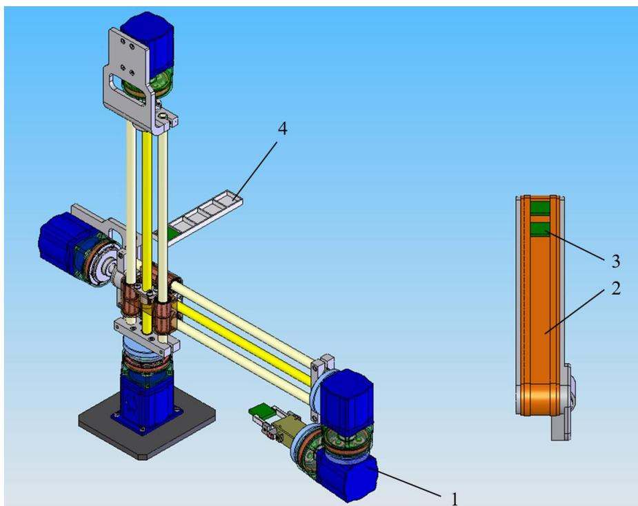
Figure 2. RTTRR small-sized industrial robot in a microprocessor packaging process
