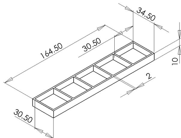
Figure 3. Partitioned tray for microprocessors
