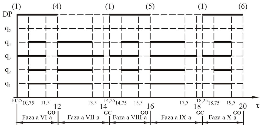
Figure 5. RTTRR robot operation cyclogram, phases VI-X
