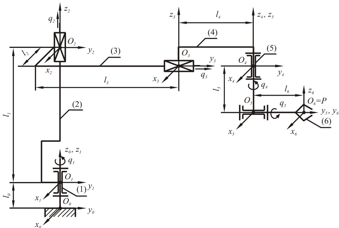
Figure 1. The kinematic sketch of RTTRR small-sized industrial robot
