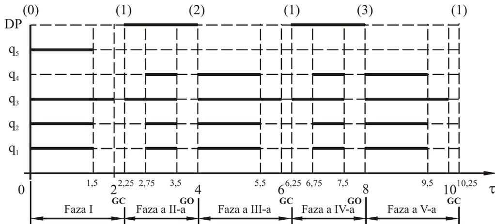
Figure 4. RTTRR robot operation cyclogram, phases I-V
