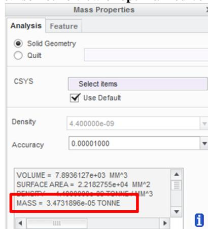
Figure 17. The weight of the optimized version.
