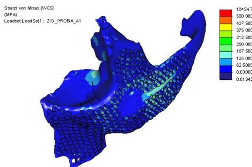
Figure 18. Von Mises tensions of optimized version.
