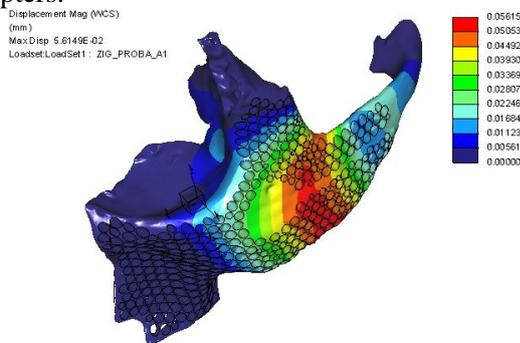
Figure 19. Deformation of the optimized version.
