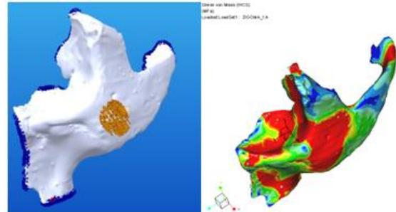
Figure 9. Test.7. Applying the force on the surface with 45 grade angle.
