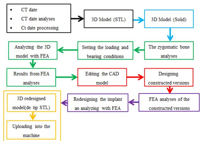
**Figure 2. Work stages of the implant created by the SLM technology**
