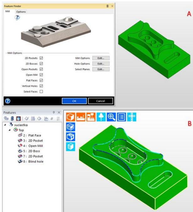
Fig. 1. Feature Finder and recognition of geometric features in Edgcam 2016.
