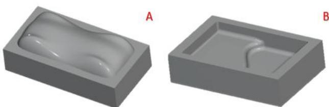
Figure 6. Sample parts A - Complex Step, B - Contured Pocket.
