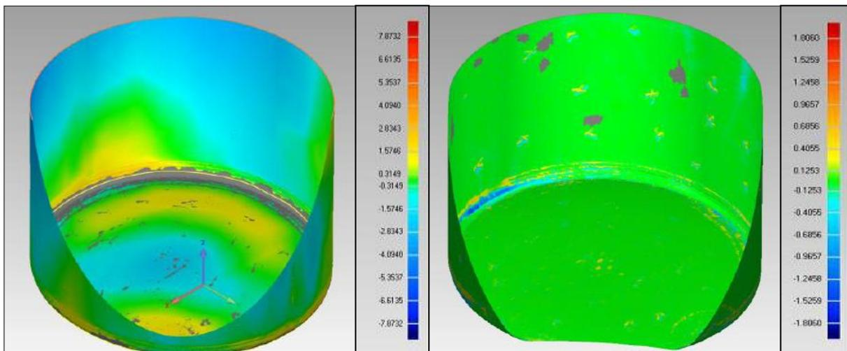
Fig. 5 a) Parametric surfaces deviation analysis, b) Exact surfaces deviation analysis
