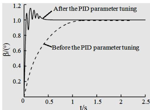
Fig 4. The system step response of opening pitch
