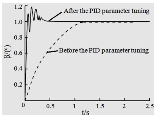
Fig 3. The system step response of closing pitch
