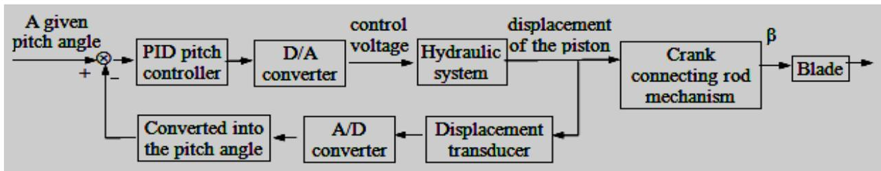
Fig 2. Control block diagram of the variable pitch control system
