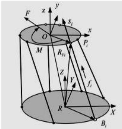
**Fig.3 Analysis on stress forces of 6-UPS surgical parallel robot.**
