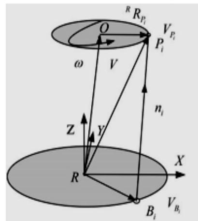
Fig.2 Velocity projection method.
