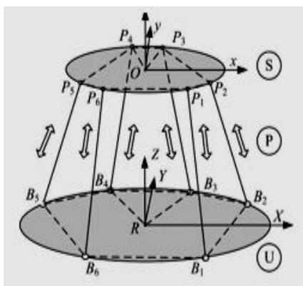
Fig.1 Structural and mechanical schematic diagrams of 6-UPS parallel robot.
