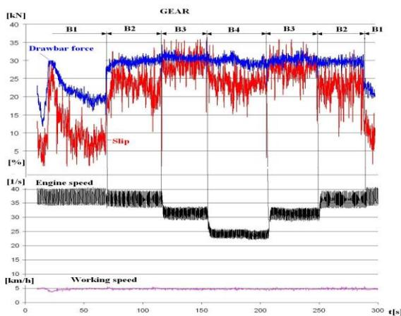
**Figure 5. Traction characteristics during underload shifting at speed controlled traction.**
