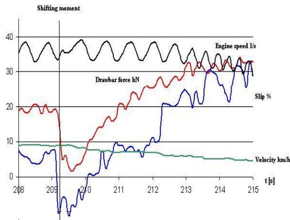
**Figure 8. Traction characteristics plotted against time at shifting from B4 to B3.**
