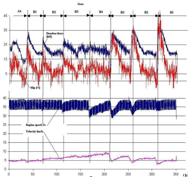
Figure 6. Traction characteristics during underload shifting at drawbar force controlled traction.
