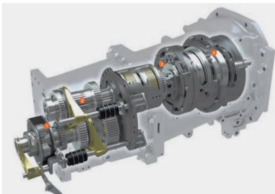
**Figure 2. The structure of the Qadrishift transmission of the tractor CLAAS.**
