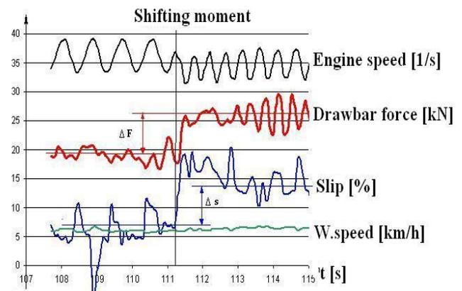
Figure 7. Traction characteristics plotted against time at shifting from B2 to B3.
