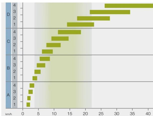
**Figure 3. Speed range covered by certain gears at an engine speed range of 1400-2100 1/min.**
