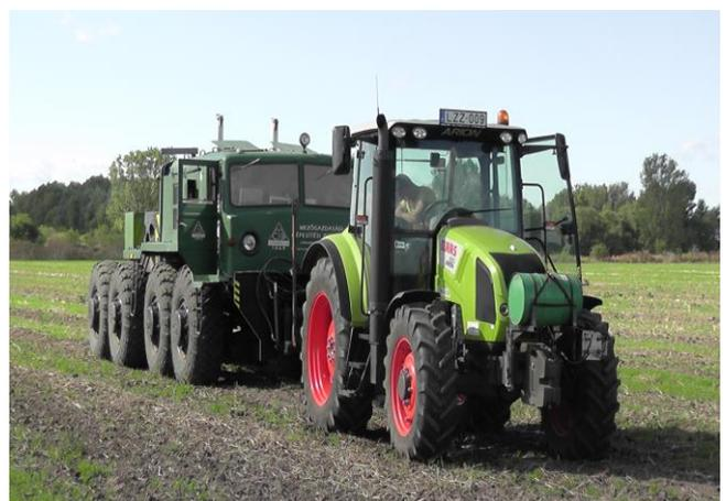
Figure 1. Tractor CLAAS and braking vehicle MAZ during field test.
