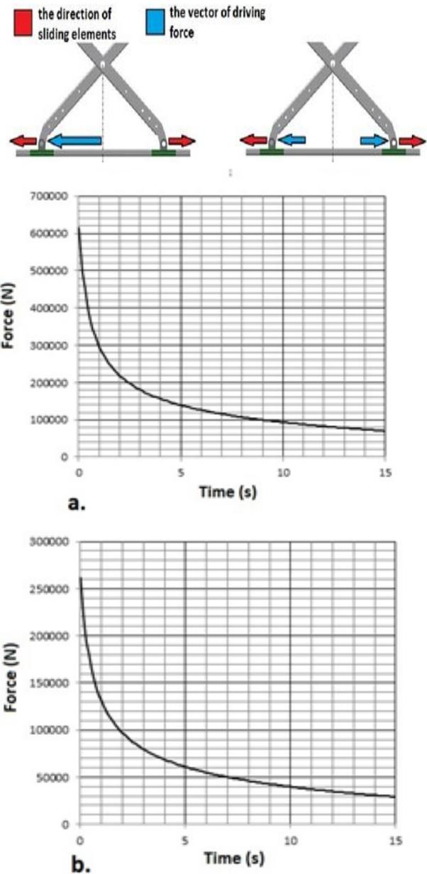
Figure 5. Comparison of asymmetric force effect (a) and symmetric force effect (b).
