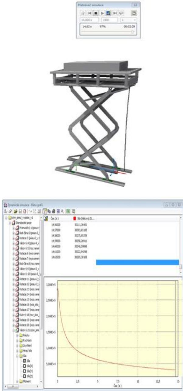
Figure 4. Dynamic simulation design of scissor mechanism (variant 1).
