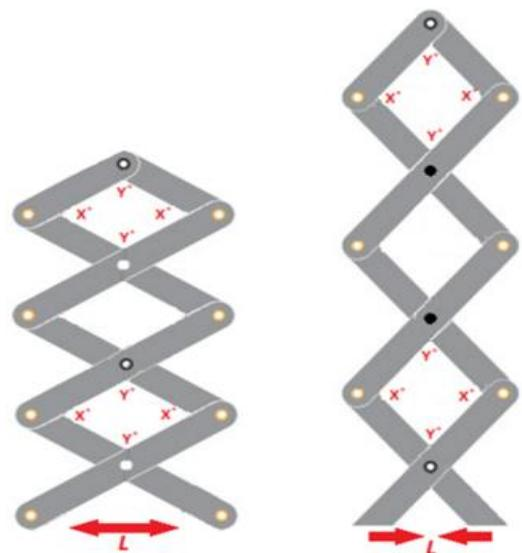
Figure 2. Schematic diagram of scissor lift [1].
