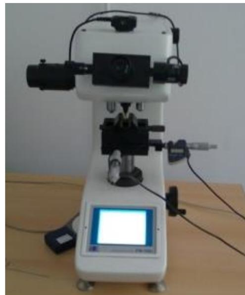
**Fig. 9. Testing the composite DUROPONT to establish hardness on a hardness microtester FM 700.**
