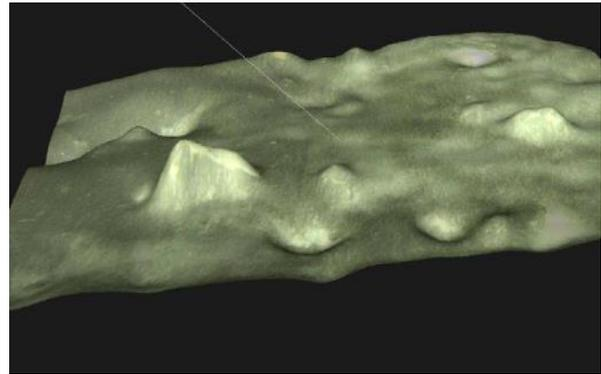
**Fig. 3. 3D microscope image, of the VALUX PLUS composite material after 6 minutes of polymerization [4].**
