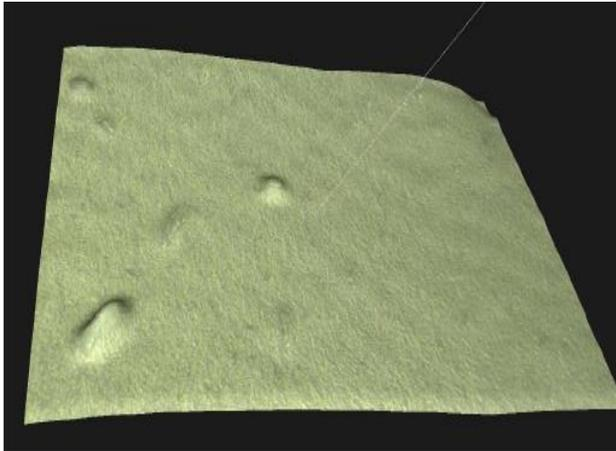
**Fig. 1. 3D microscope image of the composite material TE-ECONOM after 7 minutes of polymerisation [4].**
