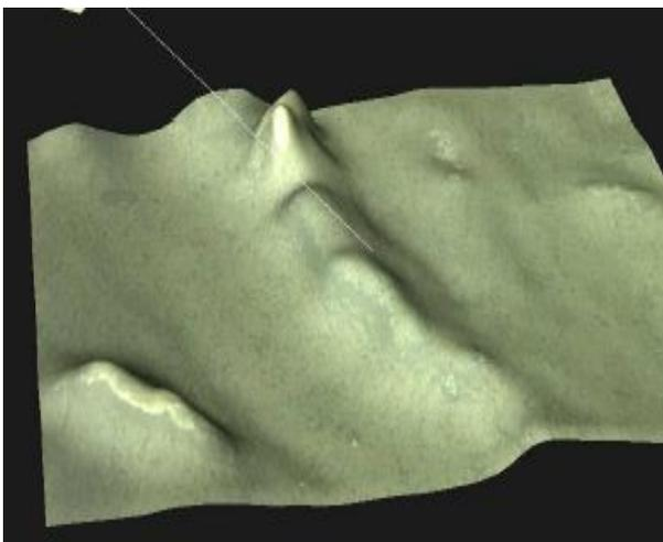
**Fig. 2. 3D microscope image, of the TE-ECONOM composite material after 9 minutes of polymerization [4].**
