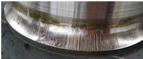
Figure 5. Inner raceway fault on 6005 bearing
