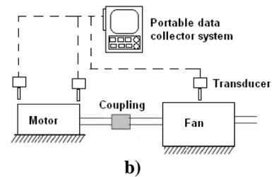
Figure 1. a) Sketch of the installation location, b) Experimental process of the fault diagnosis
