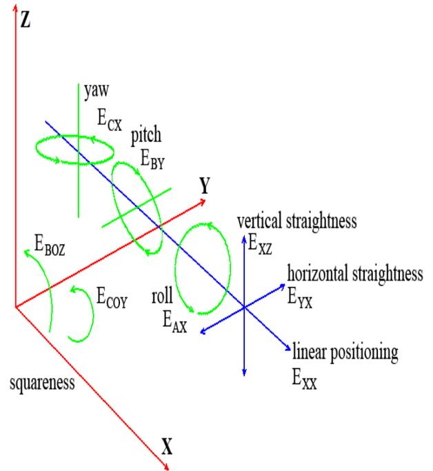
Figure 2. Errors of linear motion
