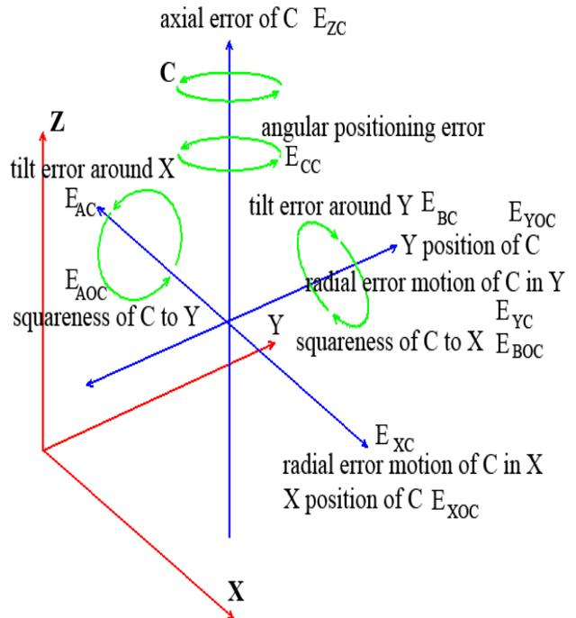
Figure 3. Errors of rotary motion
