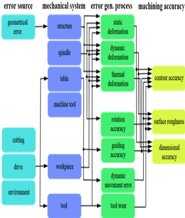
Figure 1. Machining error generation process
