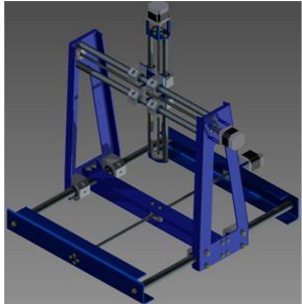
**Figure 4. Model of experimental device for practicing routines of machine tool precision measurement**
