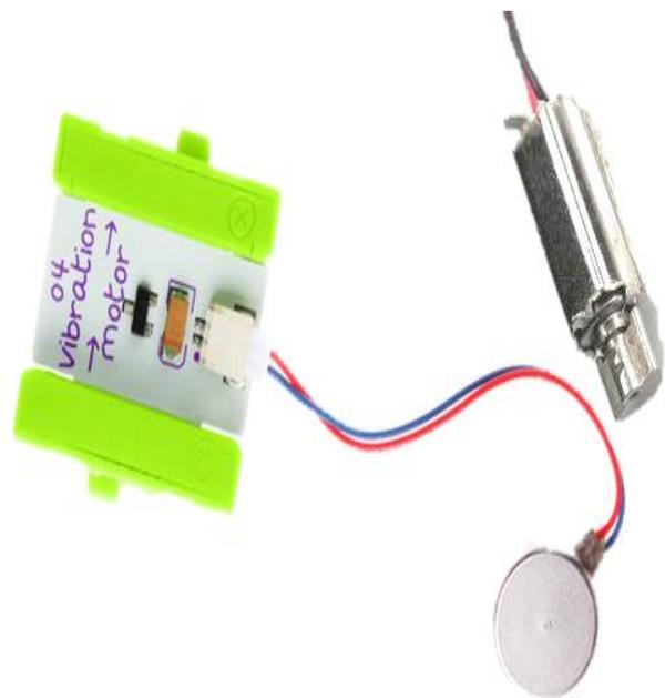
**Figure 5. Vibration motors**
