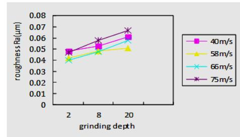
Fig. 10 roughness curve of different grinding depth.
