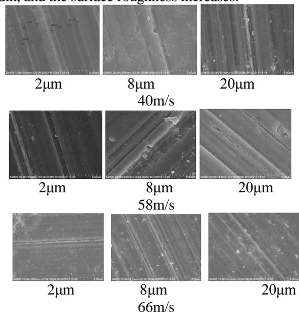
Fig. 11 The SEM examination of surface grind by W20 in different grinding depths.
