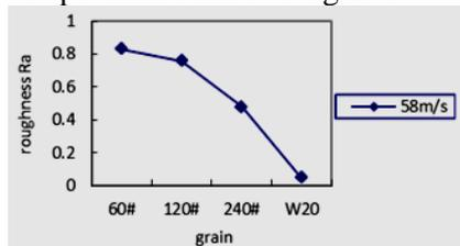
Fig. 5 Grain size affect on roughness.
