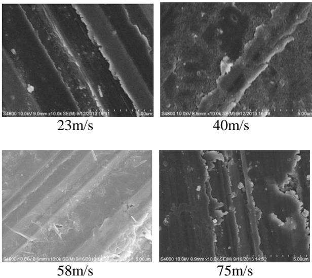
Fig. 9 grinding surface by 240# wheel at different speeds.
