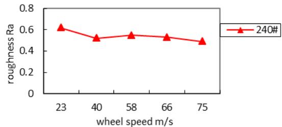
**Fig. 8 Surface roughness changing curve at different grinding wheel speed.**
