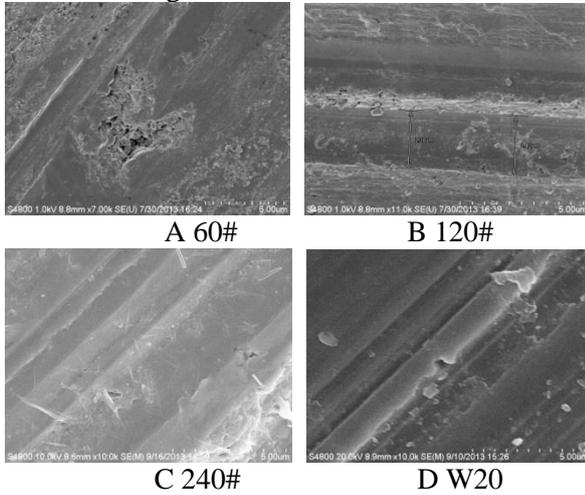
**Fig. 7 Grinding surface morphology by different grains wheel.**
