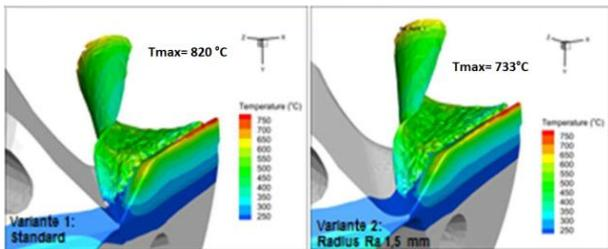
Figure 9 Heat generated by chip formation friction.
