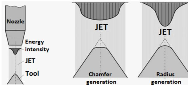
Figure 11 Influence of energy intensity of abrasive jet.
