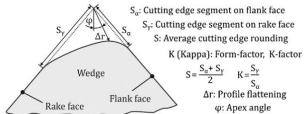
Figure 7 Form-factor methods for cutting edge characterization [8].
