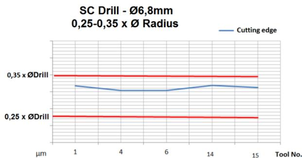
Figure 16 Edge radius for testing tools.
