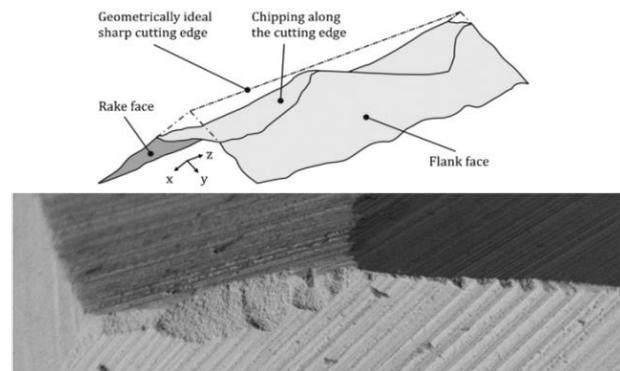
Figure 4 Cutting edge defects – after grinding.
