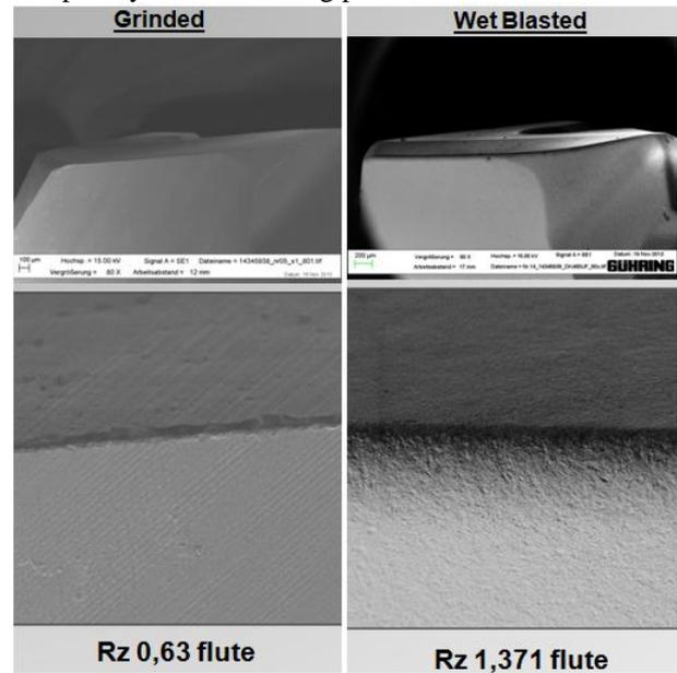
Figure 3 Cutting edge grinded and wet sand-blasted.
