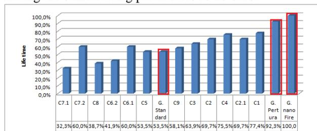
Figure 19 Drill testing – Life time in [%].
