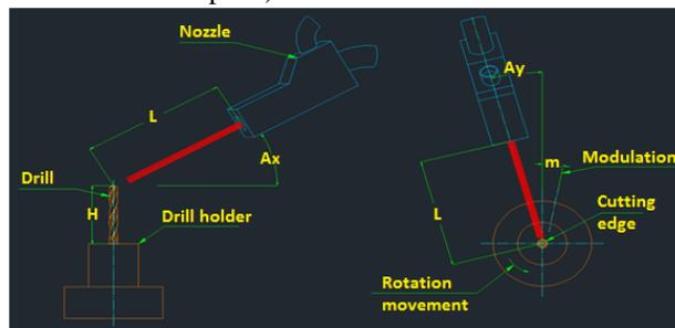
Figure 12. Geometric calibration of the nozzle.
