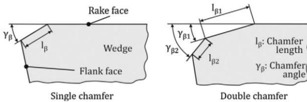
Figure 5 Cutting edge chamfer parameters.
