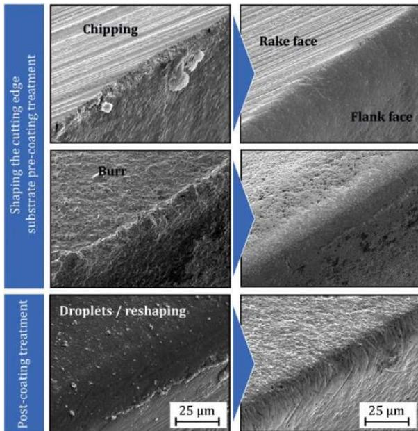
Figure 2 Main effects of the cutting edge preparation [1].
