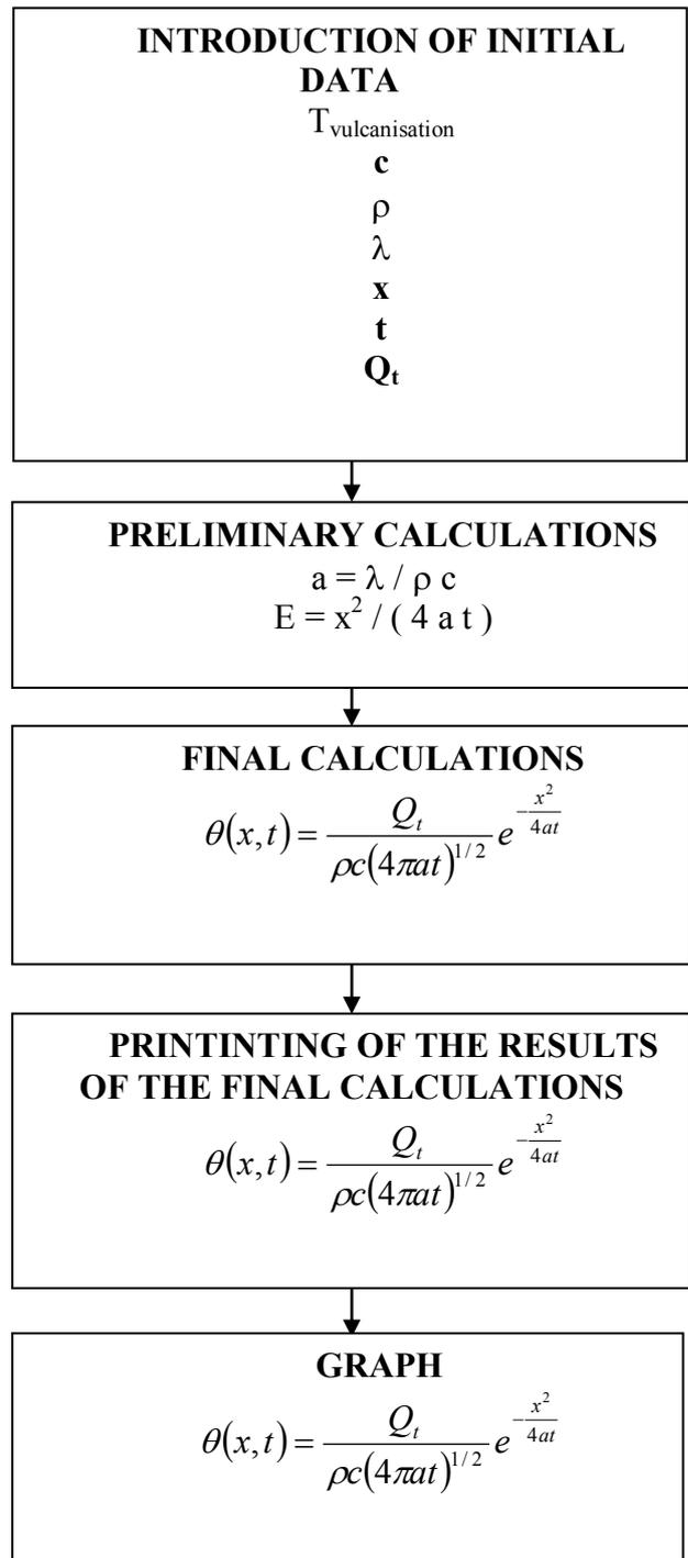
Figure 2. Structure of the calculus programme used for the modelling of the heat transfer at the vulcanisation of conveyor belts
