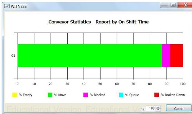
Figure 5. Report on the conveyor functioning that carries the aggregate into the oven
