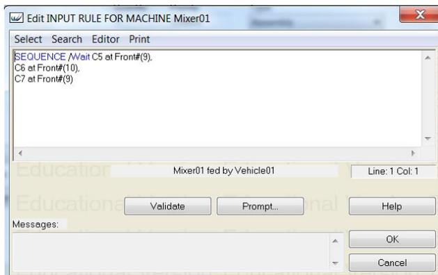
**Figure 3. Mixing rule for quantities at a structural element "Mixer01"**
