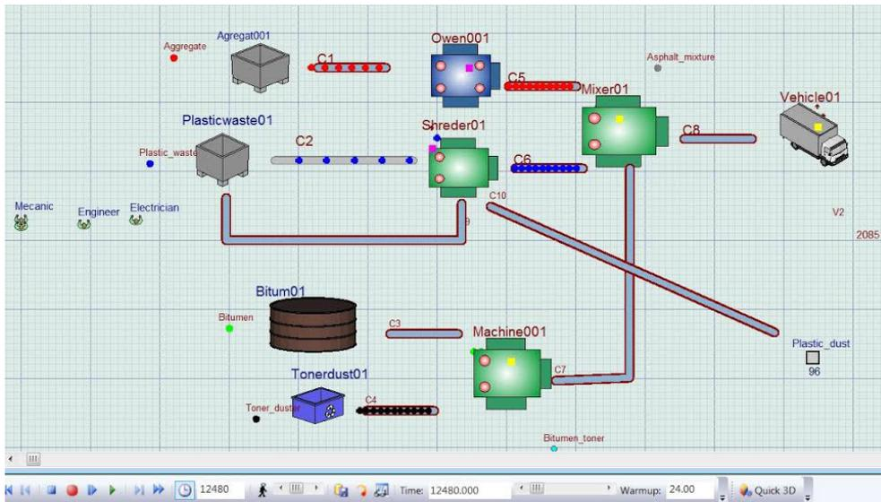
**Figure 2 Virtual model of installation for plastic waste recycling and for toner dust in the production process of asphalt mixtures in Witness 14**
