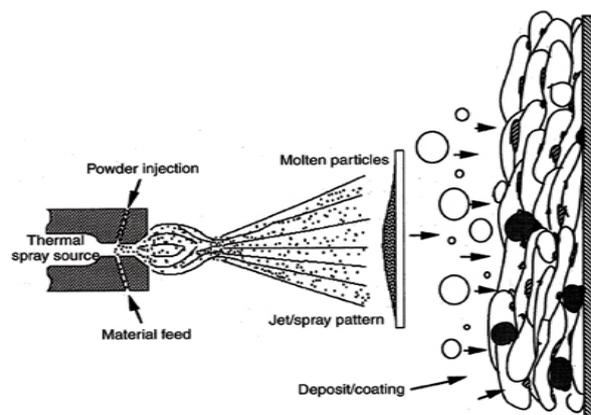
**Figure 1. Schematic representation of the thermal spray process flow and layer build-up**
