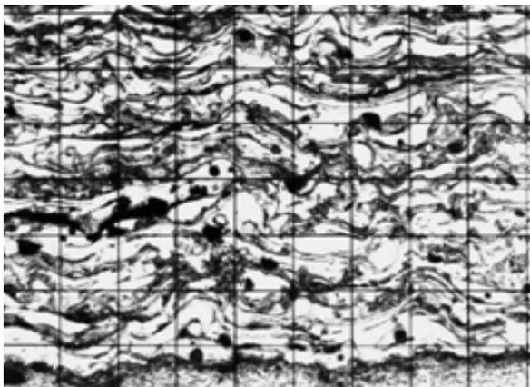
Figure 3. Metallographic structure of 40C130 coating
