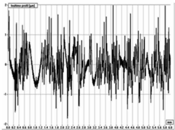
grinded surface roughness profile (b.)
