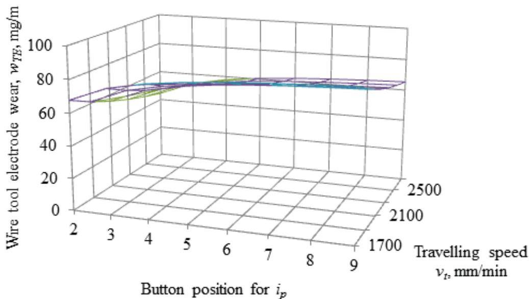
Figure 4: Influence exerted by current intensity  $i_p$  and travelling speed  $v_t$  on wire tool electrode wear  $w_{TE}$
