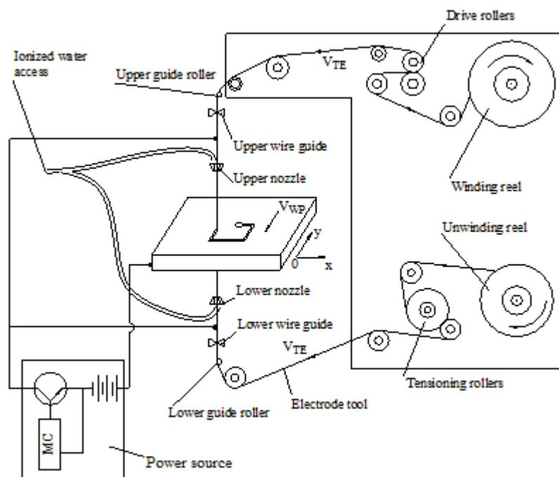
Figure 1. Machining scheme in case of wire electrical discharge machining
