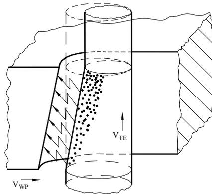
Figure 2. Erosion process that affects the wire tool electrode in the work zone
