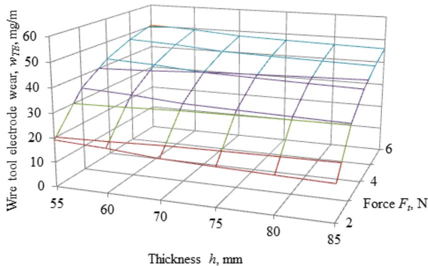
Figure 3: Influence exerted by test piece thickness  $h$  and tensile force  $F_t$  on wire tool electrode wear  $w_{TE}$
