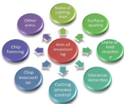
Figure 12. Aim of monitoring the cutting process
