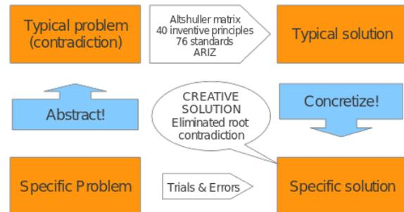
Figure 15. Schematic of TRIZ method
