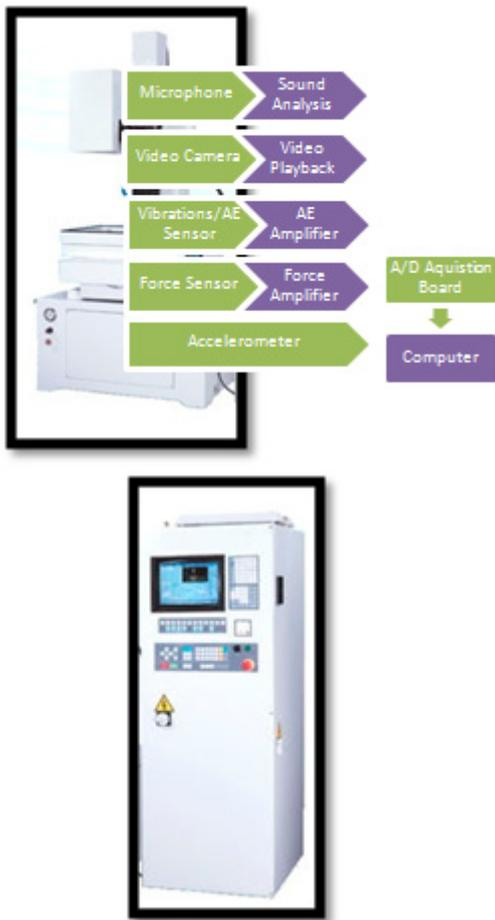
Figure 11. Reconfigurable drill monitoring system
