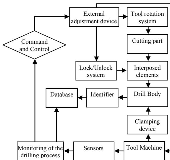
Figure 17. General model of a feasible constructive variant of an intelligent drill
