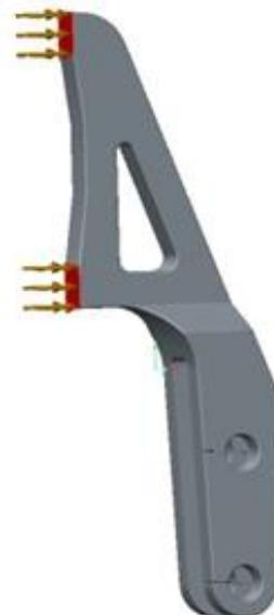
**Figure 3. Loading surfaces for clamping prismatic parts.**
